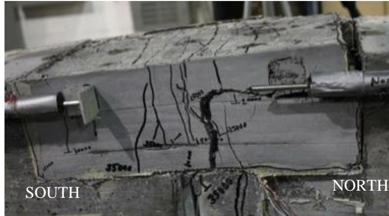
Figure 17. Side view of UHPC pocket in specimen U-6-6-I-E after failure showing the effect of prying
