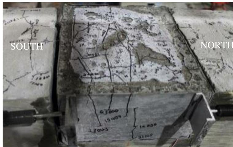
Figure 16. Interface separation and splitting cracks seen in pocket.
