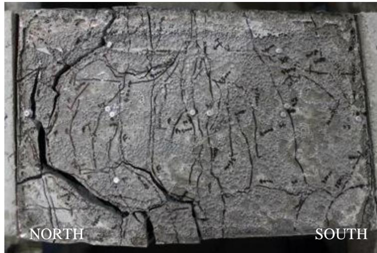
Figure 15. Large cracks at end of reinforcement due to reinforcing bar pull out.
