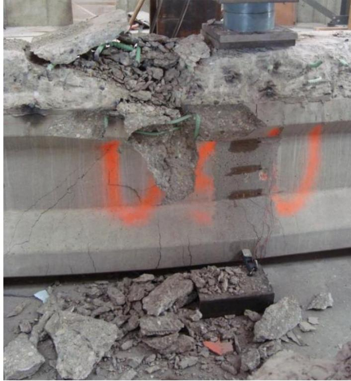
Fig. 6 Girder 1 Midspan Test, Flexural Failure
