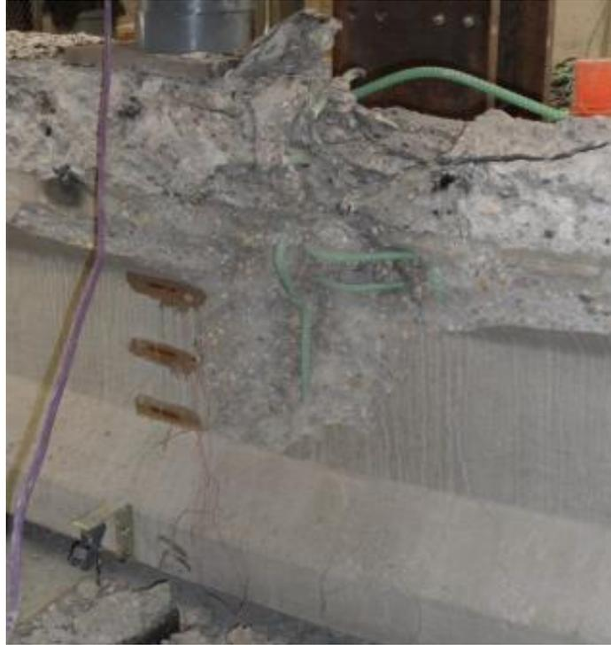
Fig. 11 G4-4HB Crushing near Applied Load
