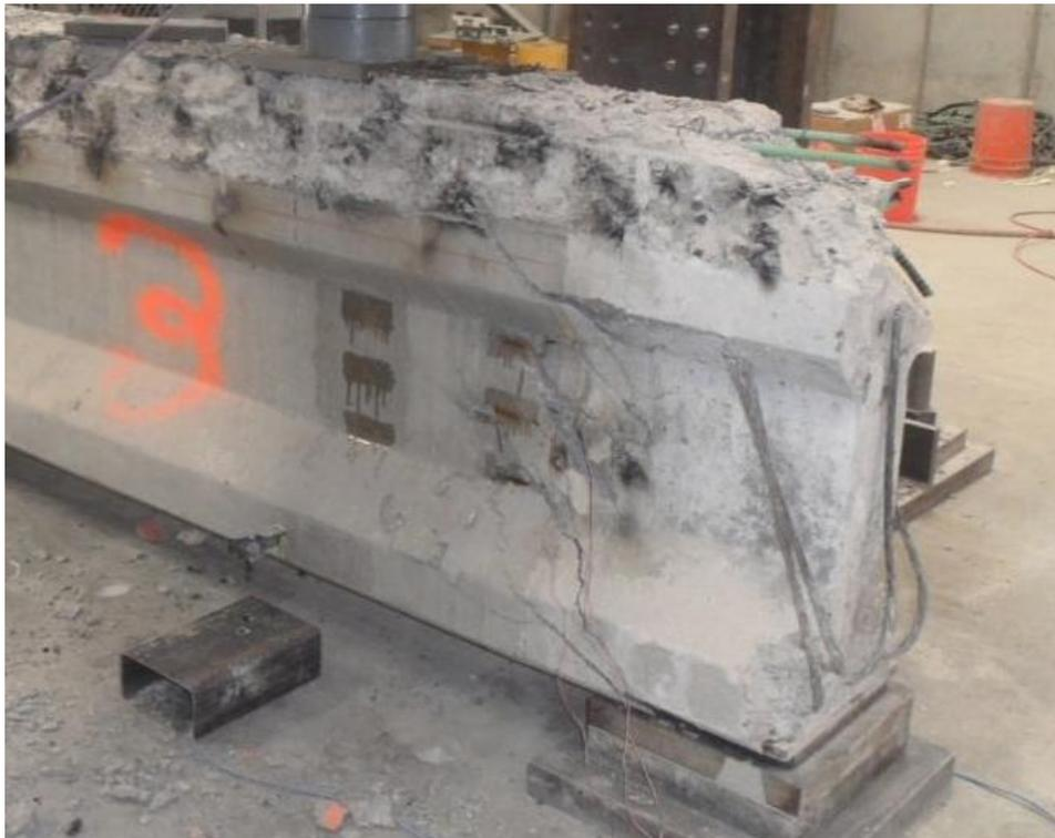
Fig. 8 Failure Cracking the 1H Test of Girder 2
