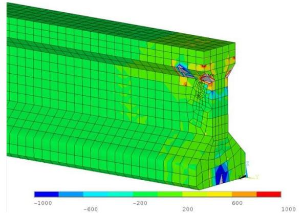
Fig 17. Principle Stress Contour Plot for Bracket Lift (psi)
