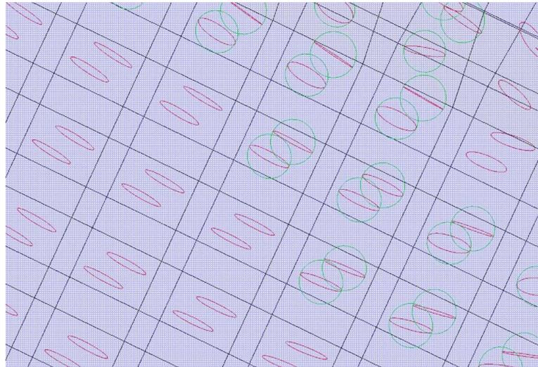
Fig. 13 Sample ANSYS Solid65 Element Cracking Results
