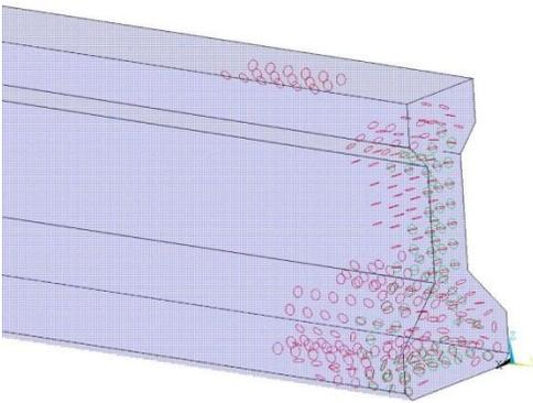
Fig.18 Cracking Plot for Bottom Flange Lift
