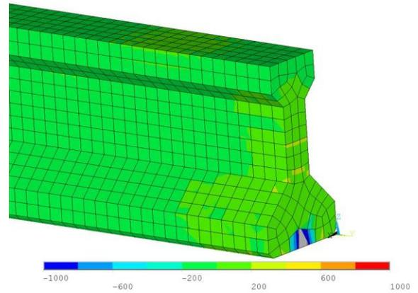
Fig. 19 Principle Stress Contour Plot for Bottom Flange Lift (psi)
