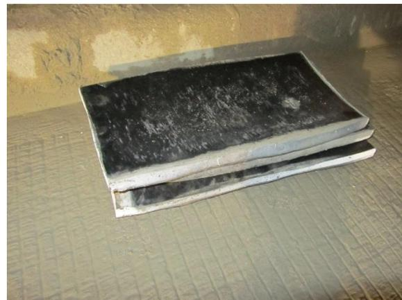
Fig. 2 Deteriorated Elastomeric Bearing Pads
