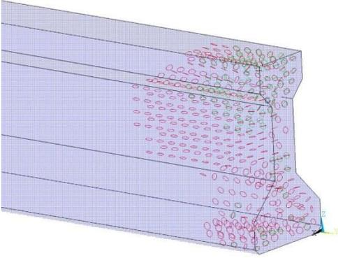
Fig. 14 Cracking Plot for Timber Lift
