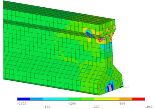
Fig. 15 Principle Stress Contour Plot for Timber Lift (psi)
