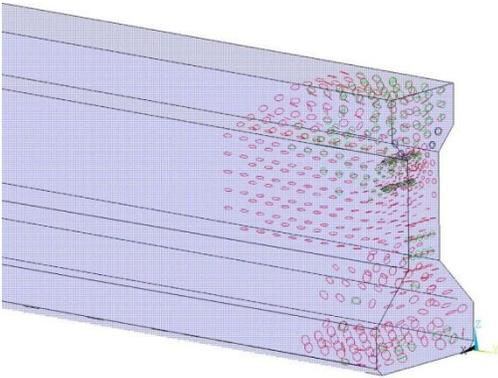
Fig 16. Cracking Plot for Bracket Lift
