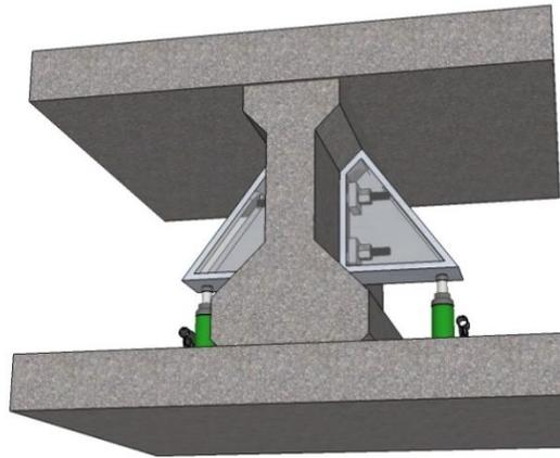
Fig. 9 Lifting with Steel Brackets
