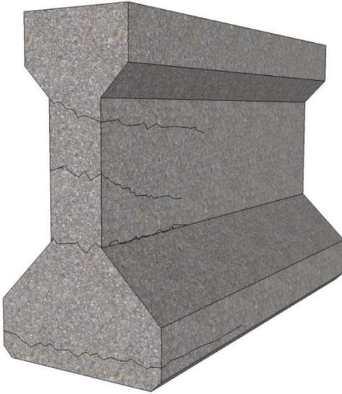
Fig 10. Typical Anchorage Zone Cracking
