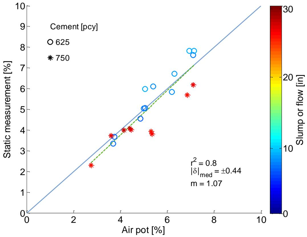
Figure 7: Static measurements versus pressure meter readings
