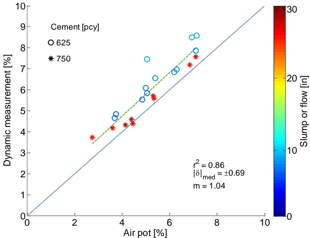
Figure 8: Dynamic measurements versus pressure meter readings
