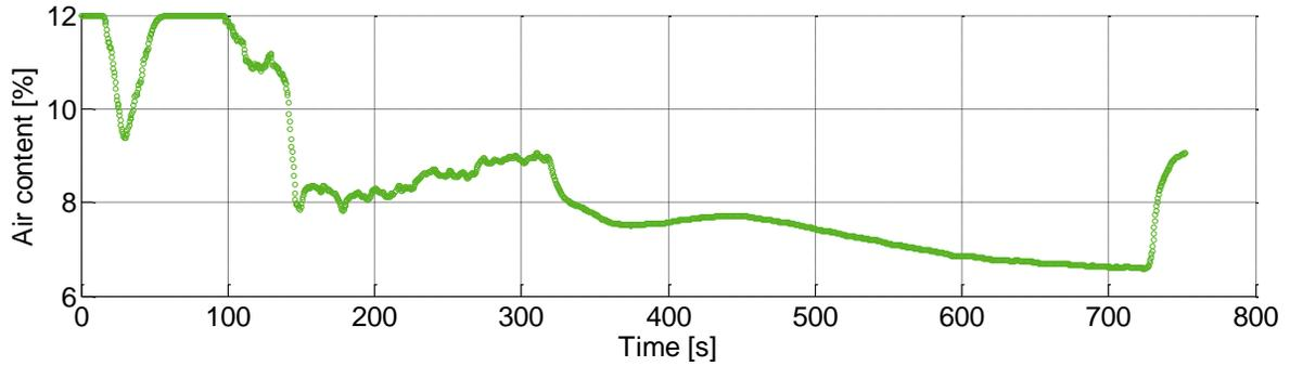
Figure 12: Real-time output from precast plant mixer
