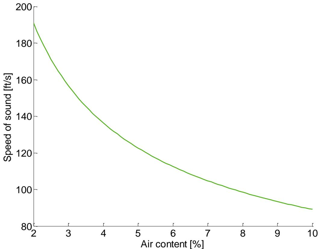
Figure 1: Wood's simplified model for plastic concrete
