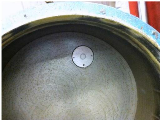
Figure 2: Sensor installed in laboratory pan mixer
