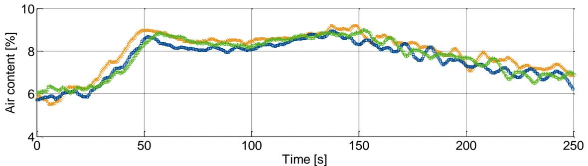
Figure 4: Repeatability of air measurement system
