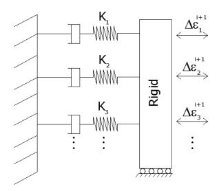
Fig. 1 - 1-D Parallel Spring Model
