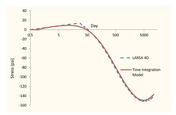
Fig. 5 - Comparison of Stress Development over Time in Topping Concrete between LARSA 4D and Time Integration Model (Positive is Concrete Tension)
