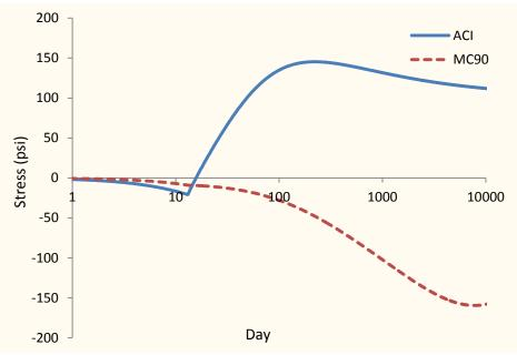
Fig. 8 - Comparison of Stress Development over Time in Topping Concrete between ACI 209R and MC 90 (Positive is Concrete Tension)
