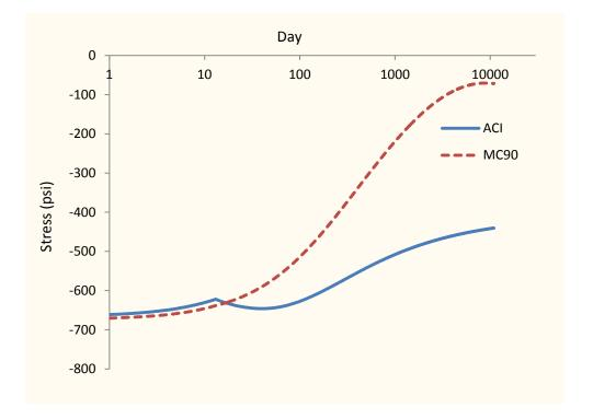
Fig. 6 - Comparison of Stress Development over Time in Pile Cap Beam between ACI 209R and MC 90 (Positive is Concrete Tension)
