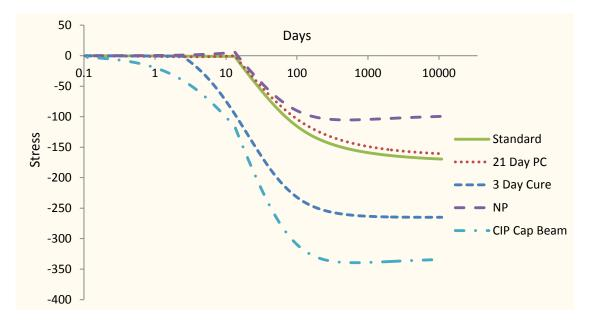
Fig. 11 - Stress Development over Time in Deck Panel for Different Construction Conditions (Positive is Concrete Tension)
