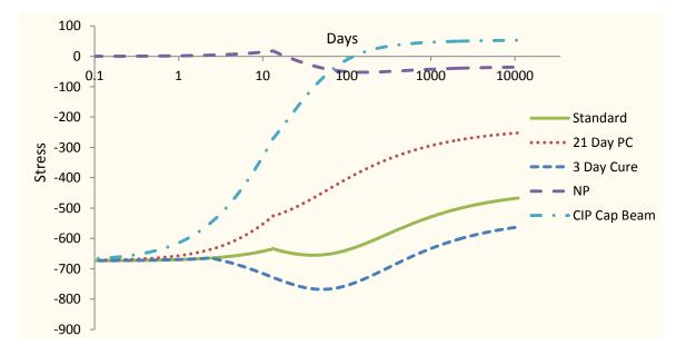
Fig. 12 - Stress Development over Time in Cap Beam for Different Construction Conditions (Positive is Concrete Tension)
