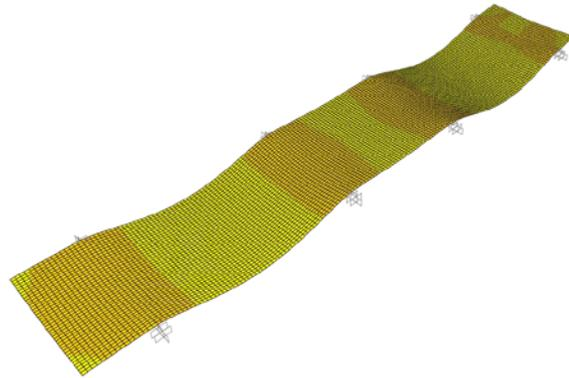
Figure 17. Maximum bottom tensile panel stress of 79 psi in the panel and 217 psi at supports.
