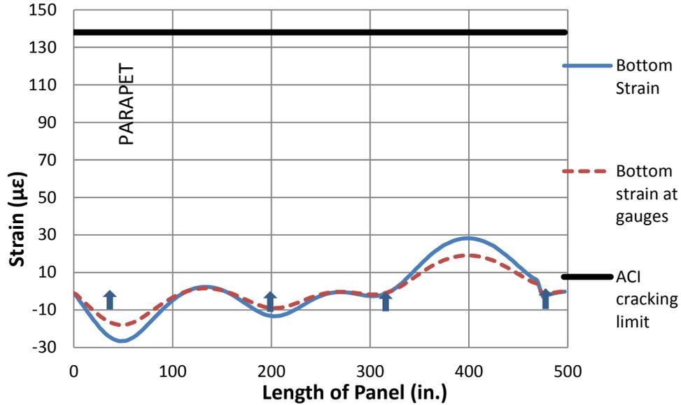
Figure 29. Midline strains of bottom of deck panel while lifting- Lift 2
