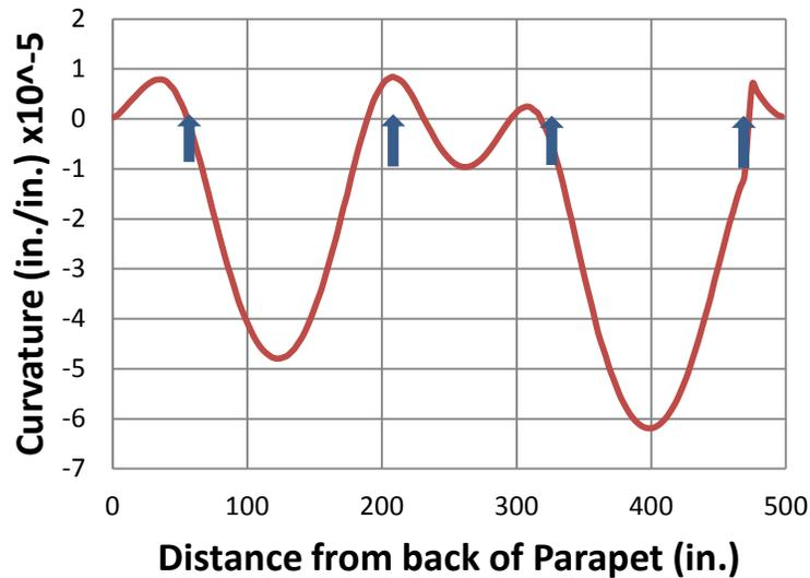
Figure 25. Curvature for panel lifting without the parapet- Lift 1
