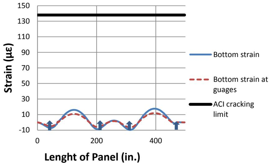
Figure 18. Mid-line bottom tensile strains of panel while on ground
