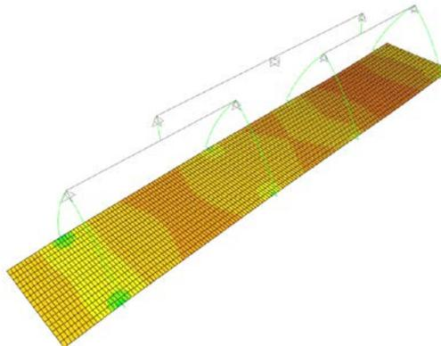
Figure 26. Maximum tensile stress of 128 psi at the top of deck panel while lifting- Lift 2
