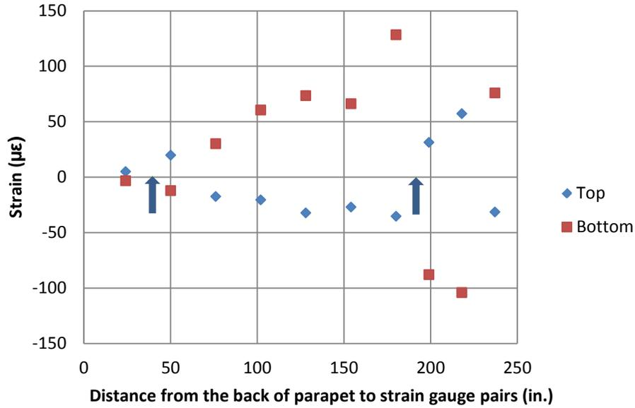
Figure 10. Strain Profile for P25 during its first lift removing it from the formwork
