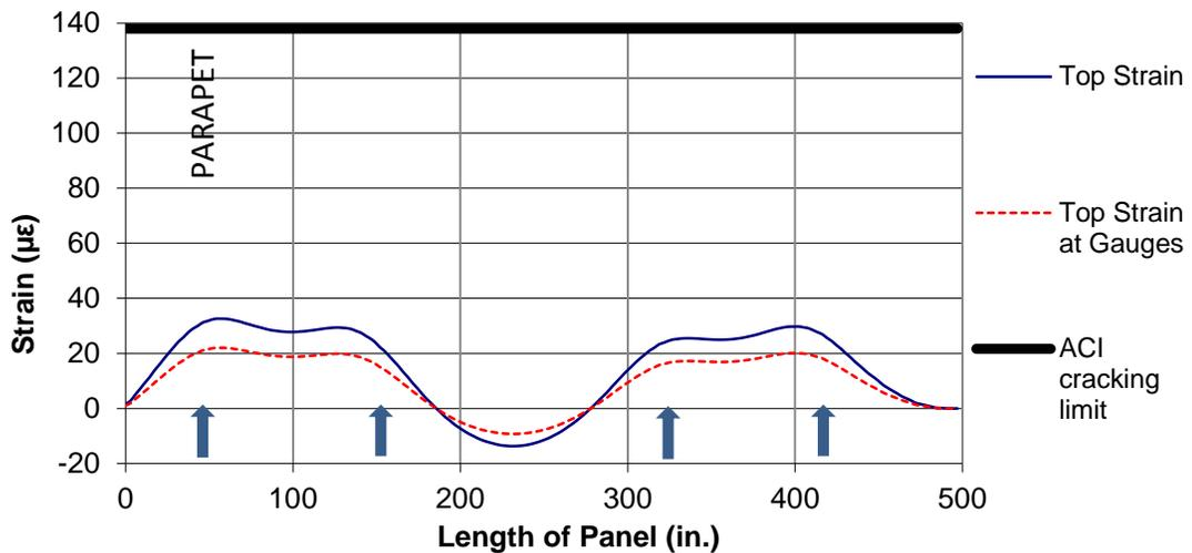
Figure 33. Mid-line top strain with parapet- Lift 3
