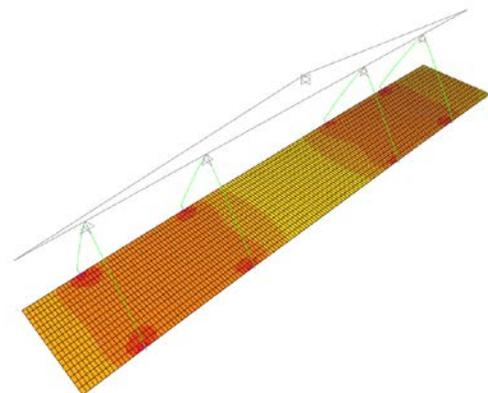
Figure 34. Maximum Bottom Stress panel with parapet is -144 psi (compression)-Lift 3
