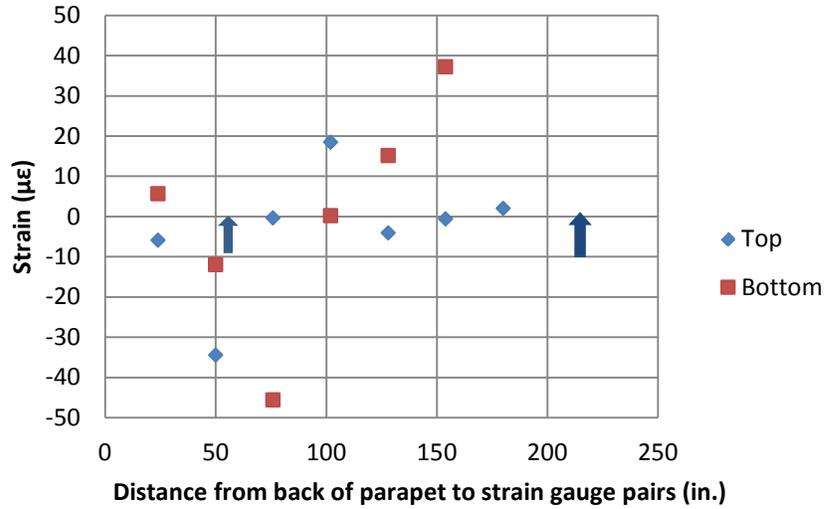
Figure 13. Strain profile for EP3 during its third lift
