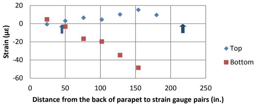
Figure 11. Strain Profile for panel EP3 during its second lift
