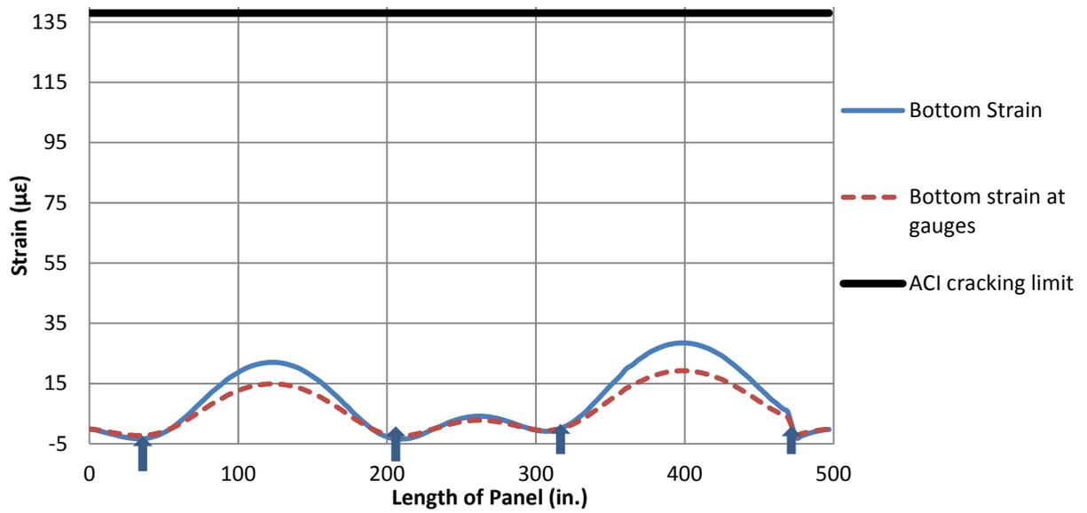
Figure 22. Mid-line bottom strain without parapet- Lift 1
