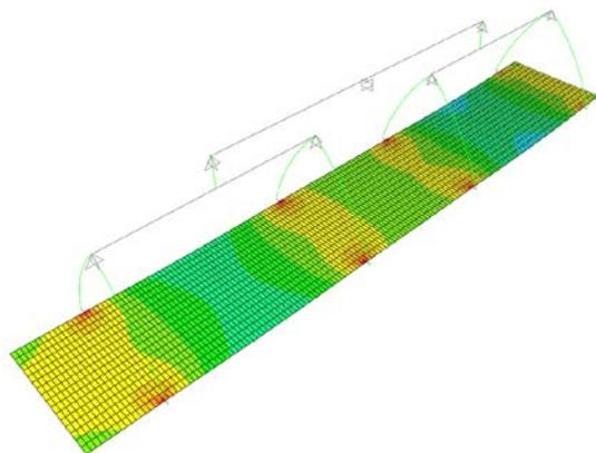
Figure 21. Maximum tensile stress of 129 psi at the bottom of deck panel while lifting- Lift 1
