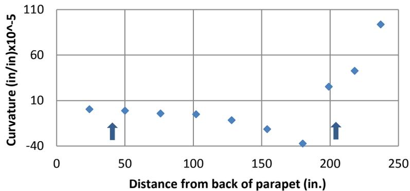
Figure 14. Curvature diagram from experimental results EP3 Lift 1
