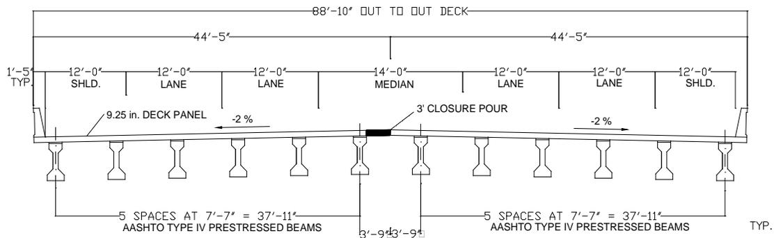
Figure 1: Elevation of Beaver Creek Bridge showing deck and girders.
