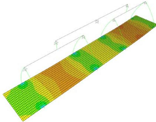
Figure 19. Maximum tensile stress of 19 psi at the top of deck panel while lifting-Lift 1
