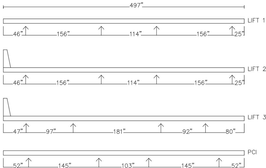
Figure 5. Lifting Point Diagram
