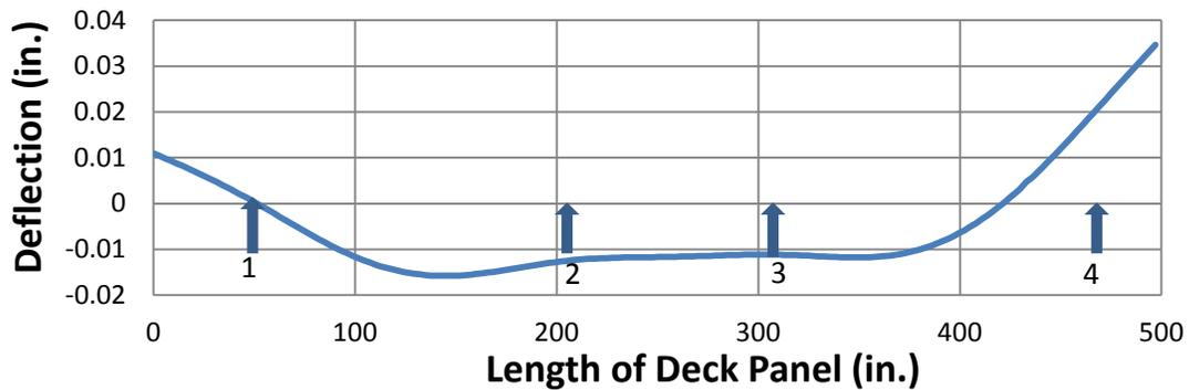
Figure 24. Midline displacement for panel lifting without the parapet- Lift 1
