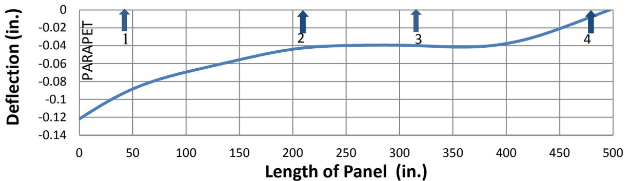
Figure 31. Midline displacement for panel lifting with the parapet-Lift 2
