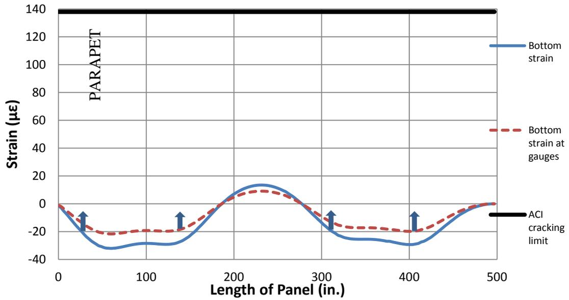
Figure 35. Mid-line bottom strain with parapet- Lift 3
