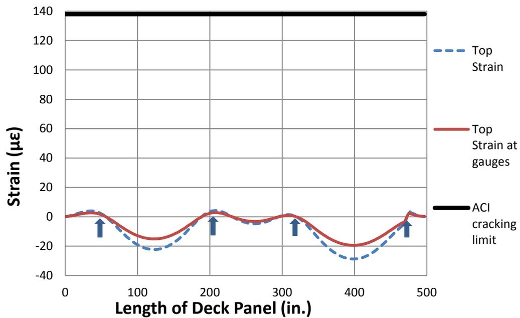
Figure 20. Mid-line top strain without parapet- Lift 1.
