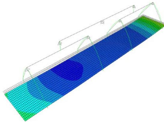
Figure 23. Deflected panel with a maximum midline deflection of 0.035 in.- Lift 1
