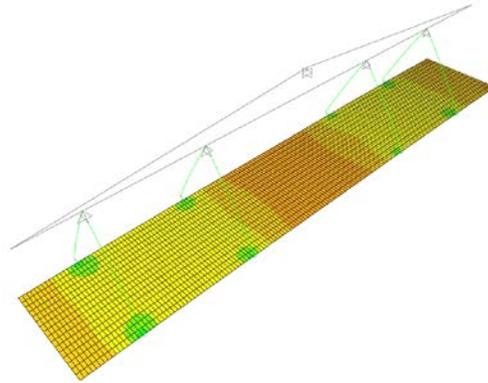
Figure 32. Maximum tensile top stress of panel with parapet while lifting is 146 psi- Lift 3
