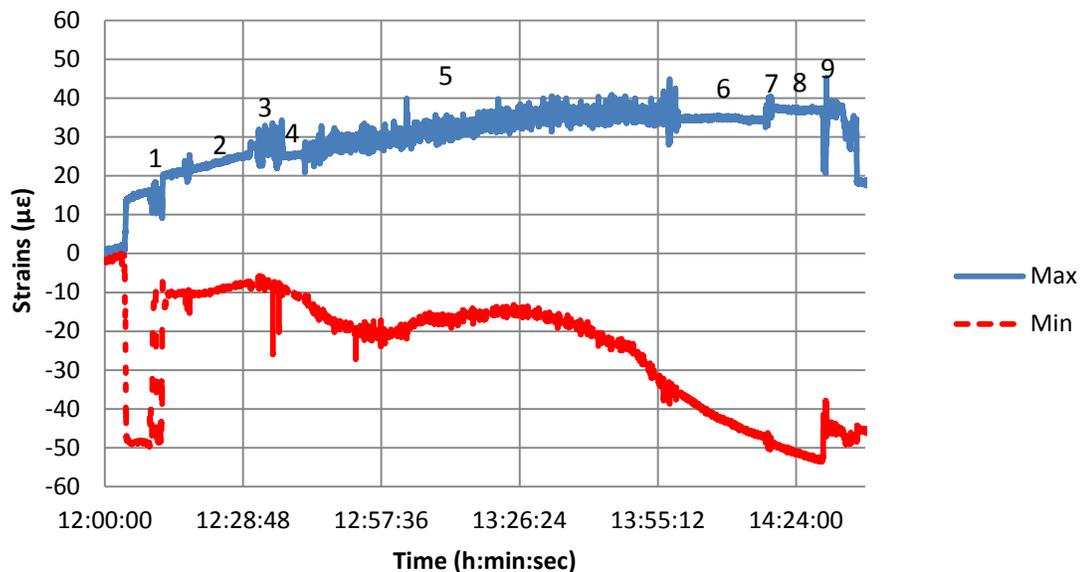
Figure 12. Maximum and minimum of all gauges during transport of panel EP3
