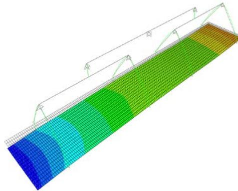
Figure 30. Deflected panel with a maximum midline deflection of -0.12 in.-Lift 2
