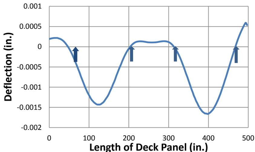
Figure 16. Midline displacement for panel sitting on the ground
