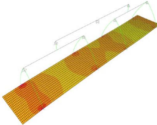
Figure 28. Maximum stress of 127 psi (tension) at the bottom of deck panel while lifting- Lift 2
