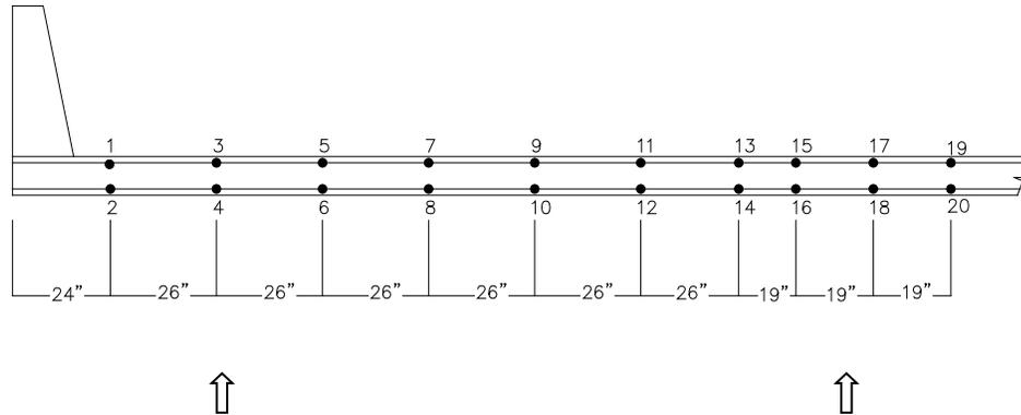
Figure 9. Electrical gauge locations for both panels and lift points located at midline of panel
