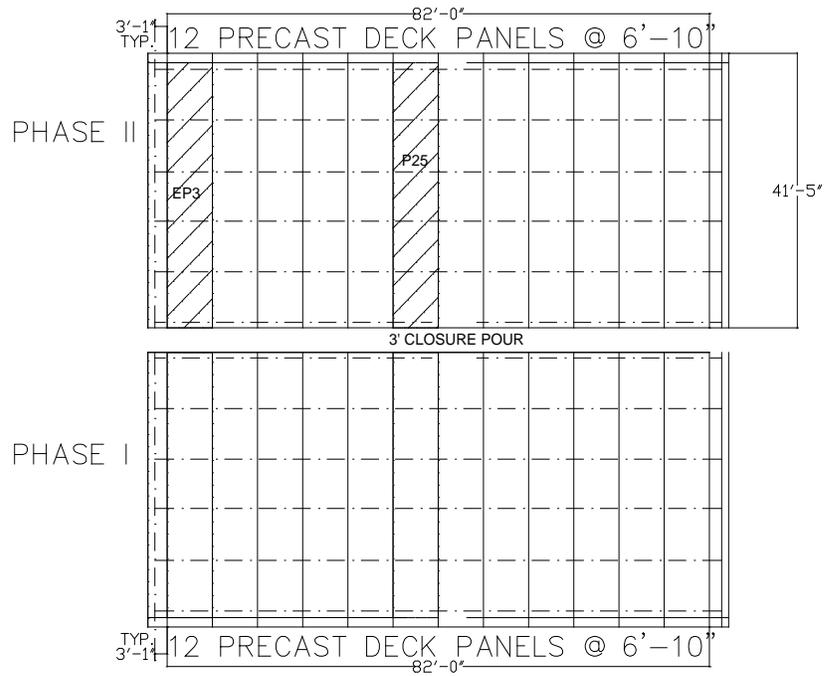
Figure 2: Plan view of Beaver Creek Bridge showing prestressed girders and deck panels.
