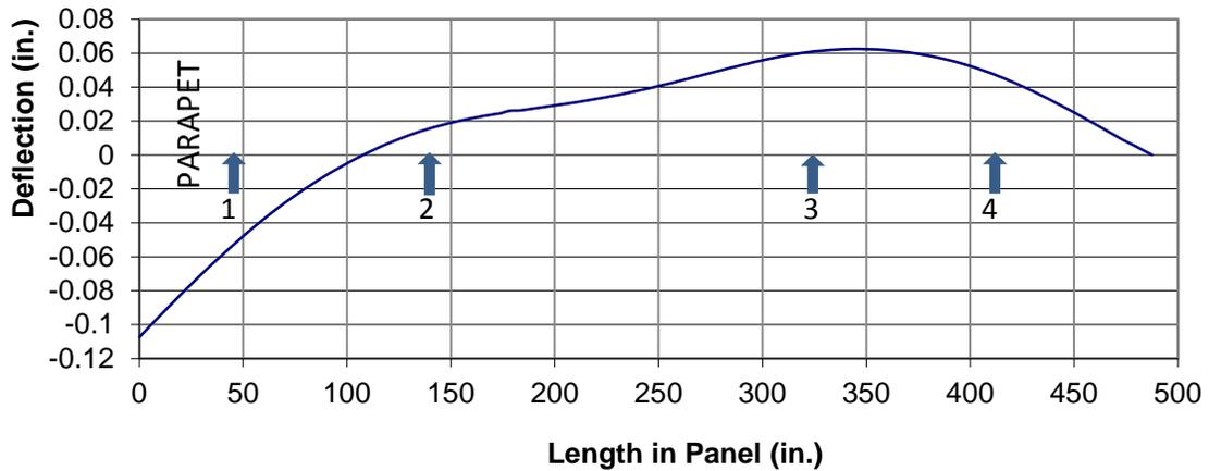
Figure 37. Deflected panel with a maximum midline deflection of -0.11 in.- Lift 3
