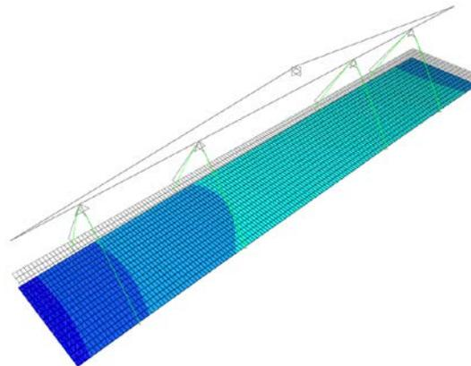
Figure 36. Deflected panel with a maximum midline deflection of -0.11 in.-Lift 3
