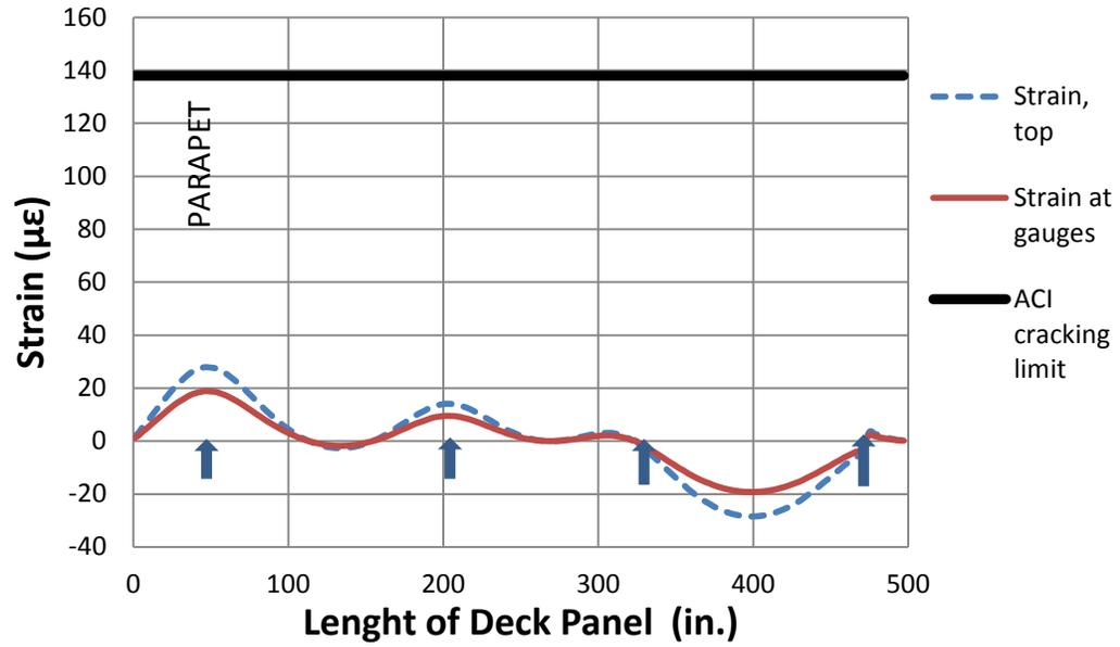
Figure 27. Midline strains of top of deck panel while lifting- Lift 2
