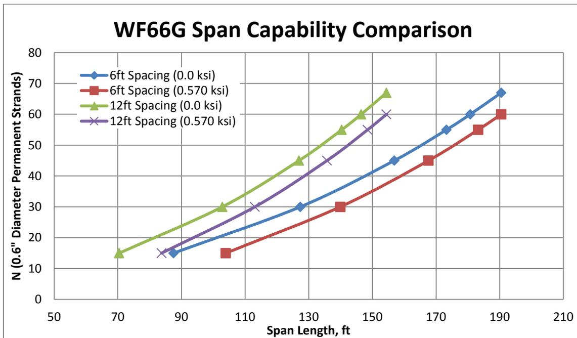
Figure 9 WF66G span capability comparison for allowable tension policy
