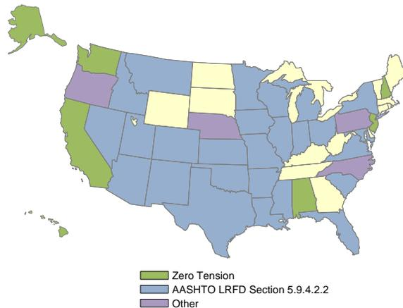
Figure 2 Survey results for Allowable Tension Design Policy
