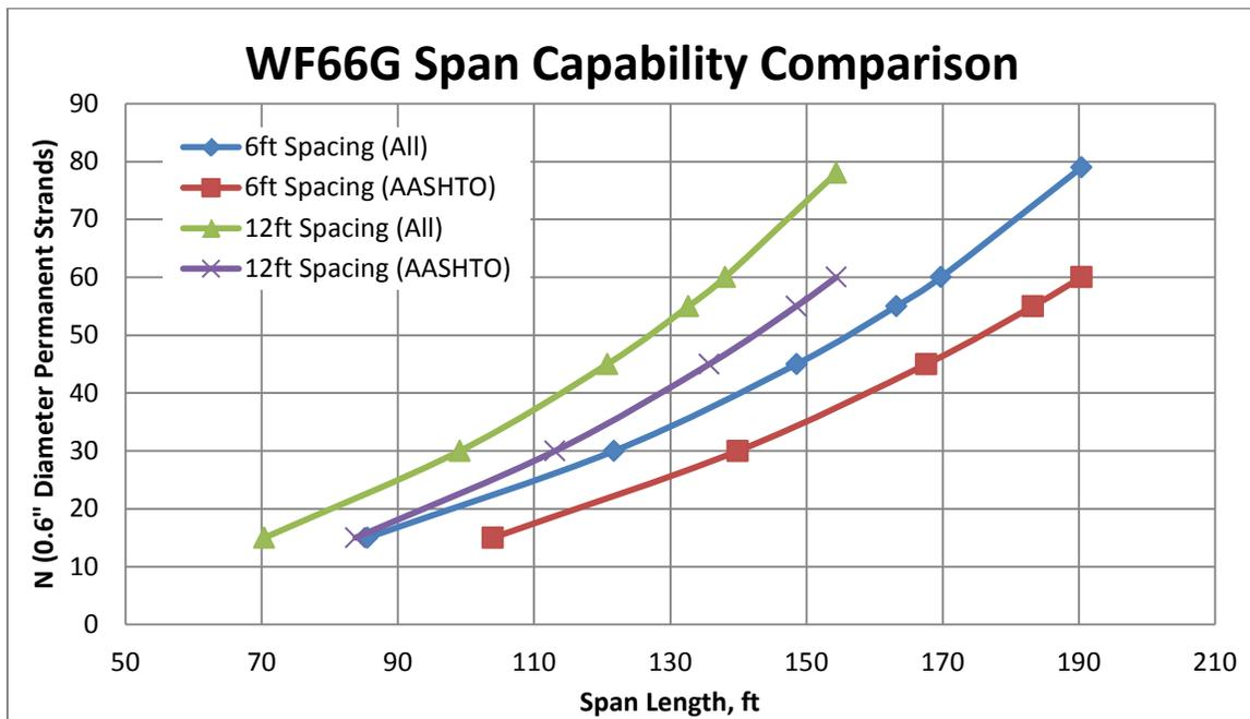
Figure 13 WF66G span capability comparison for all policies
