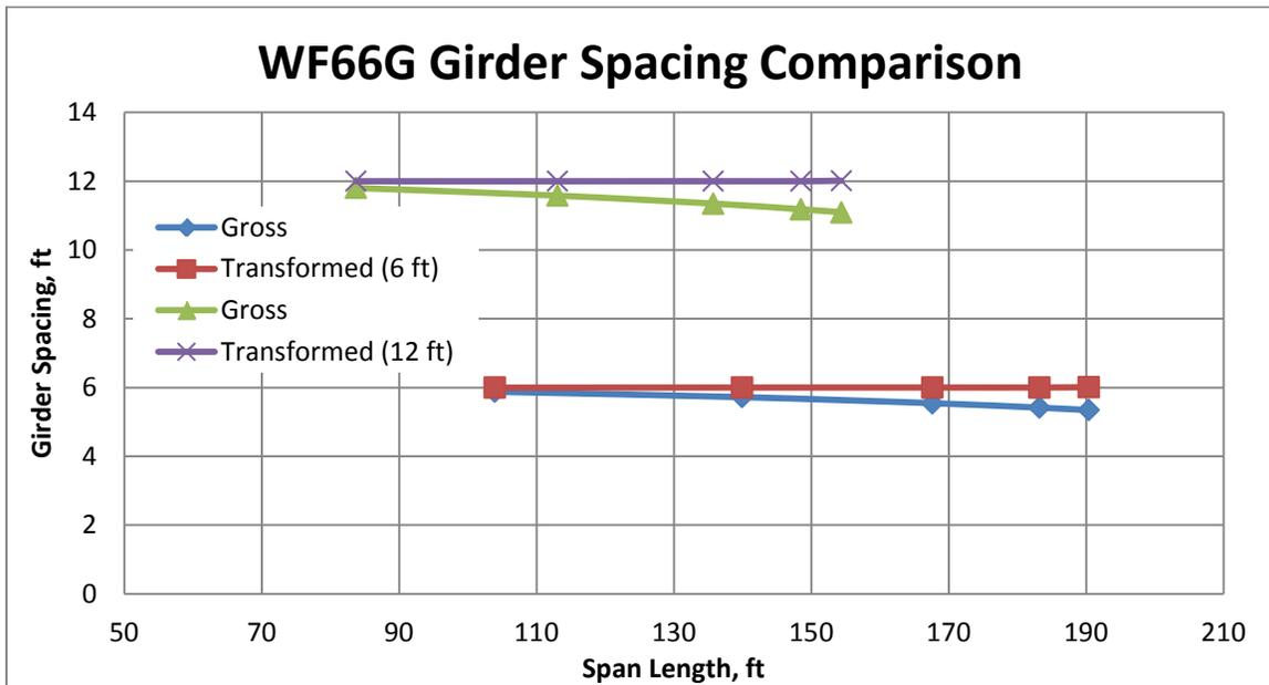
Figure 8: WF66G girder spacing comparison for section properties policy
