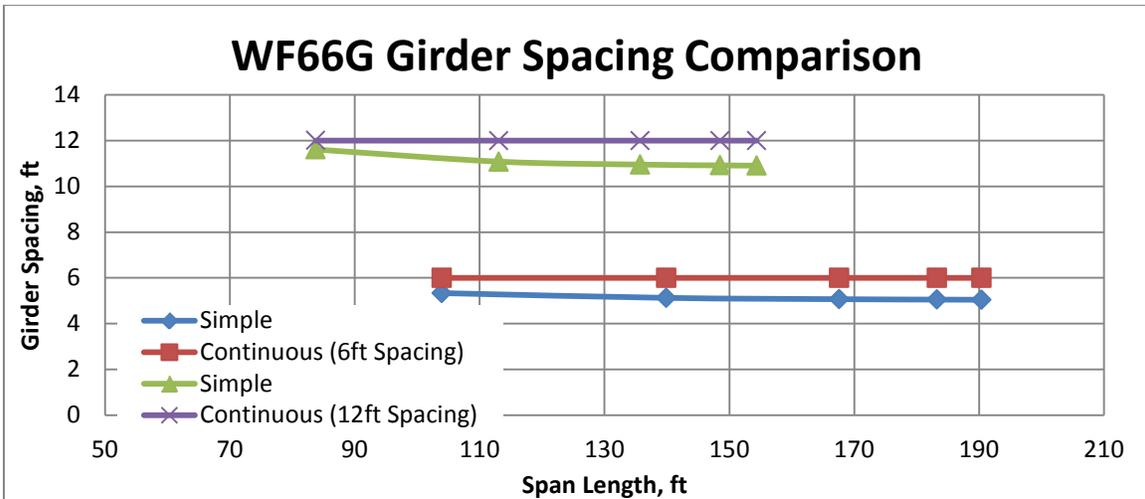
Figure 12 WF66G girder spacing comparison for continuity policy
