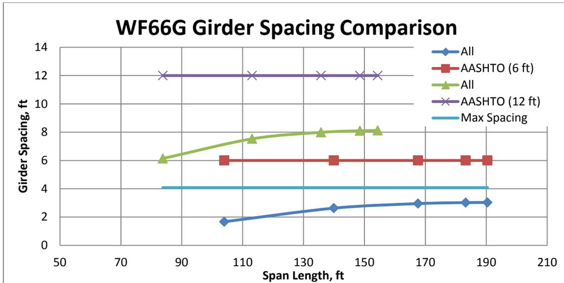
Figure 14 WF66G girder spacing comparison for all policies
