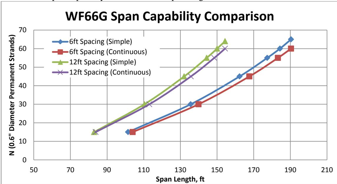
Figure 11 WF66G span capability comparison for continuity policy
