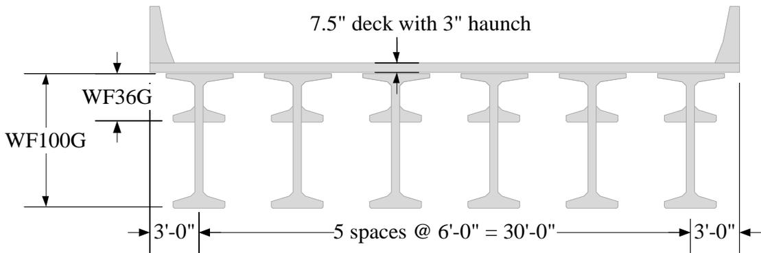
Figure 4 Bridge Section with 6 ft girder spacing.
