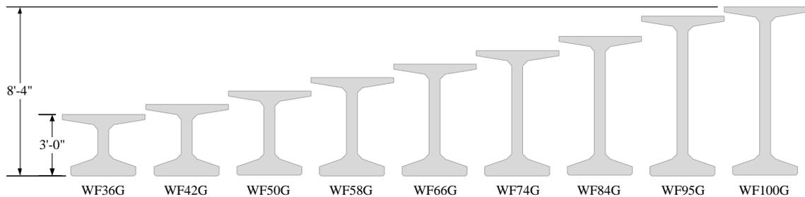
Figure 6 WSDOT WF-Series Girders
