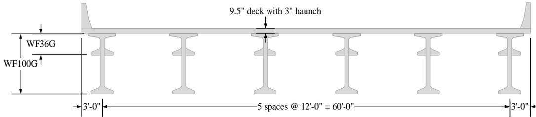
Figure 5 Bridge Section with 12 ft girder spacing.
