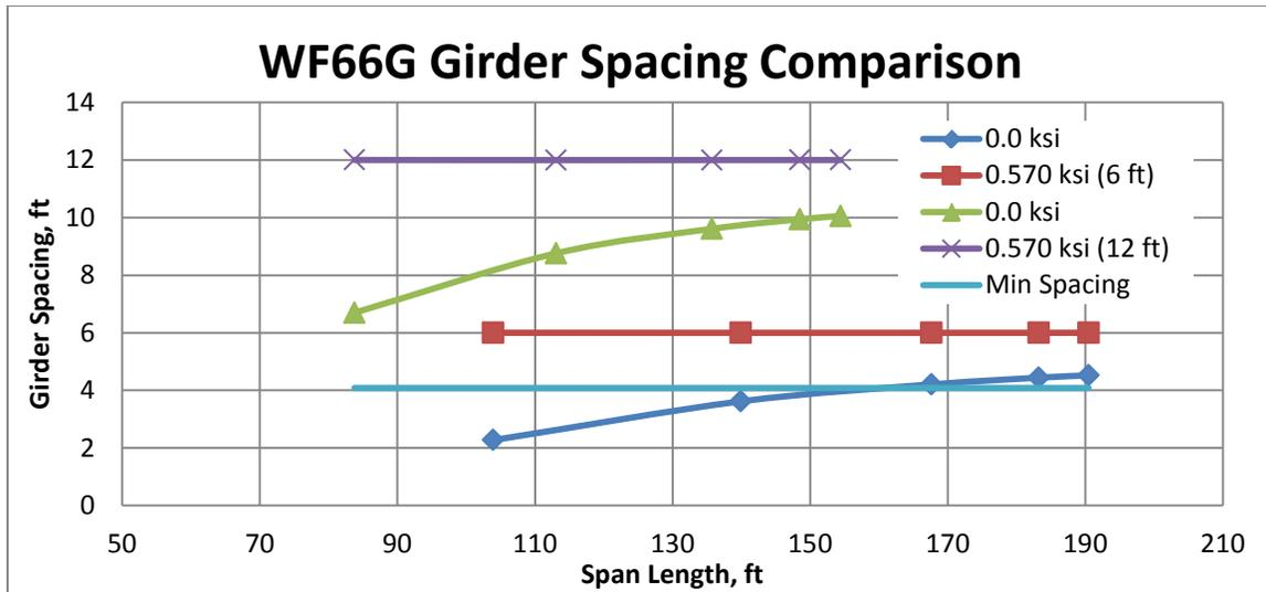
Figure 10 WF66G girder spacing comparison for allowable tension policy
