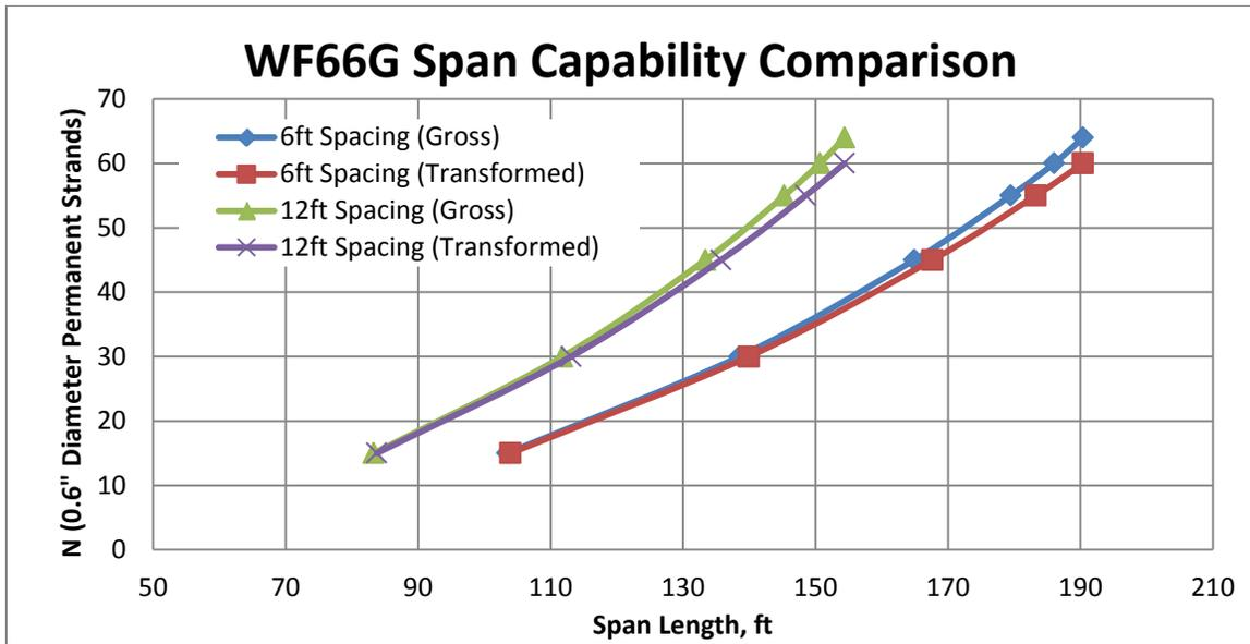
Figure 7 WF66G span capability comparison for section properties policy
