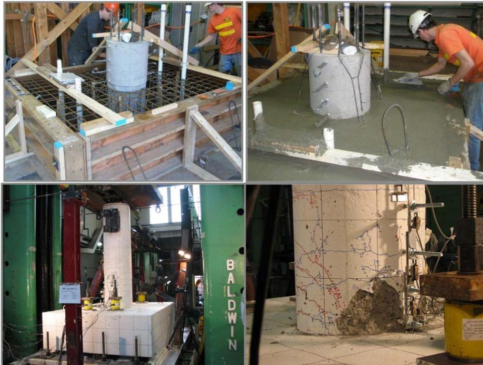
Figure 6: UW Test setups for precast column-to-footing connection
