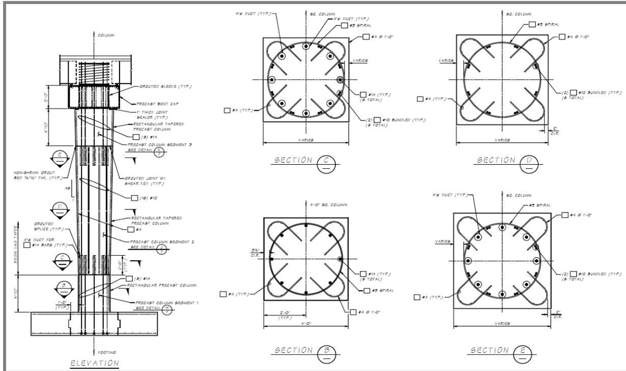
Figure 9: HFL Bridge Segmental Column Details
