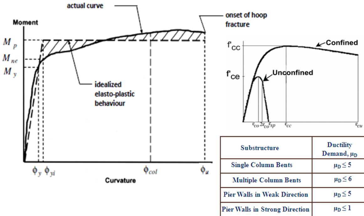
Figure 2: Stress–Strain Model, Moment–Curvature Diagram, and Ductility Demand
