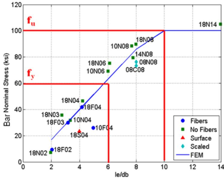
Figure 5: UW grouted Bar-Duct Pullout Test Results
