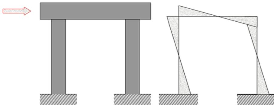
Figure 1: Moment Diagram of a Bridge Pier with Fixed Connections
