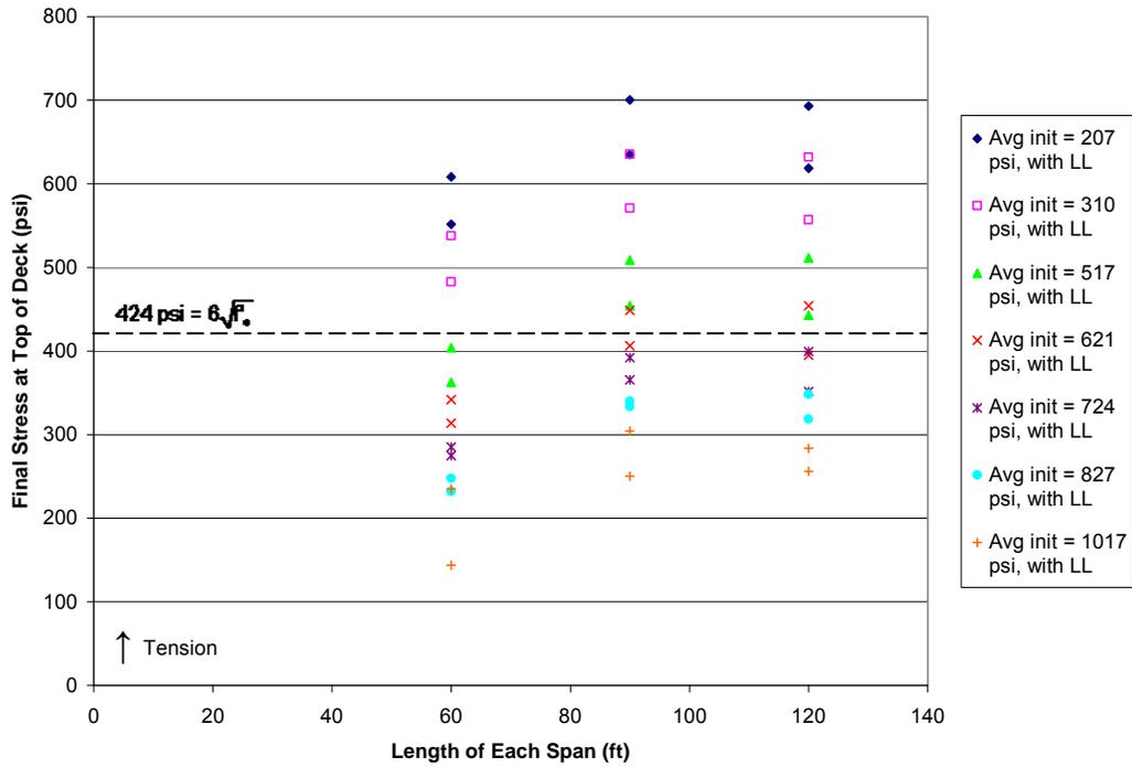
Figure 9. Final Stresses for Two-Span Continuous Steel Girder Bridges, Including Live Load
