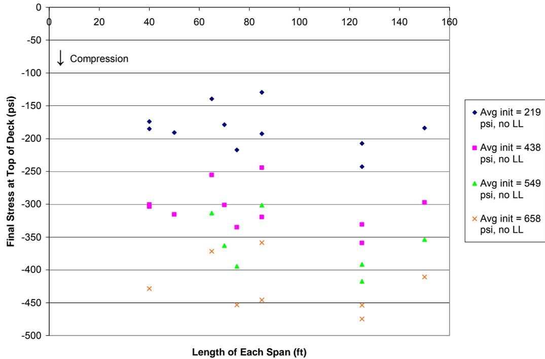
Figure 12. Final Stresses for Two-Span Continuous PCBT Girder Bridges, Not Incl. Live Load
