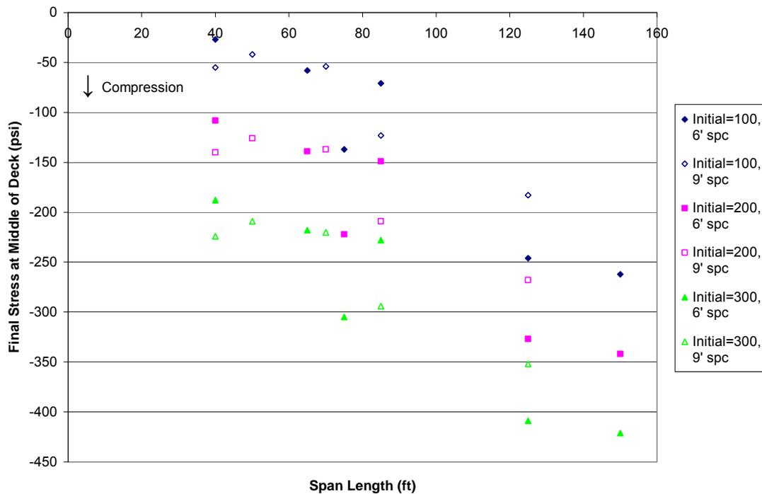
Figure 7. Final Deck Stress vs. Span Length for Simple Span PCBT Girder Models
