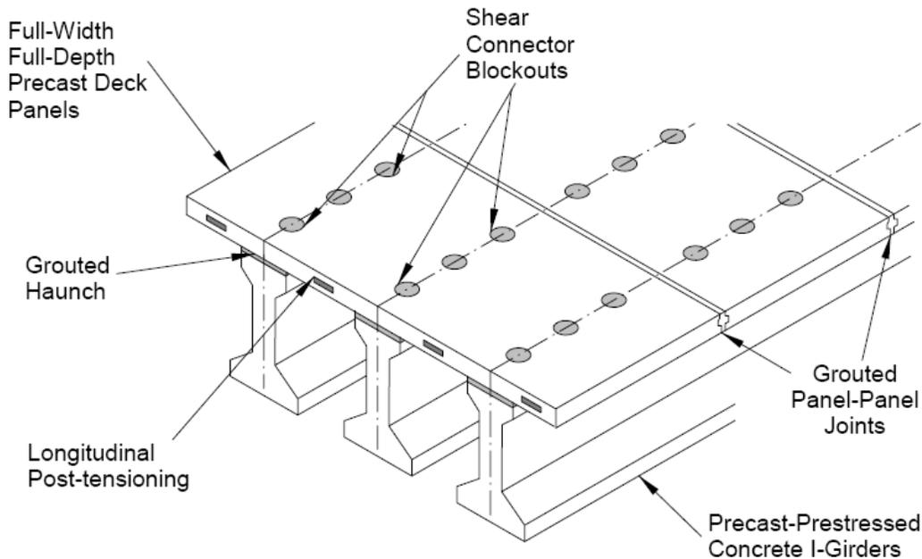
Figure 1. Precast Concrete Bridge Deck Panel System
