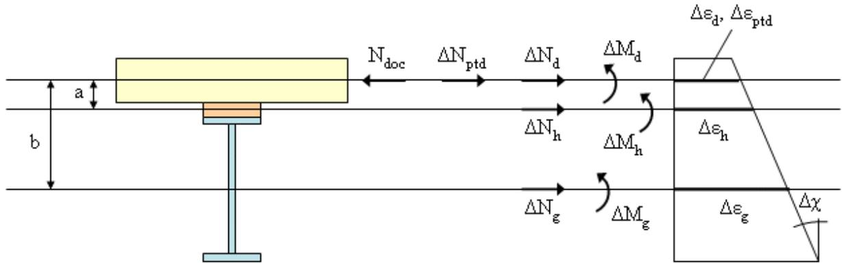
Figure 2. Initial Force and Changes Occurring in the D/SG 2 Phase
