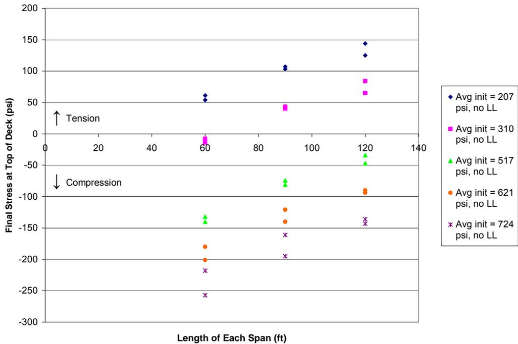
Figure 10. Final Stresses for Two-Span Continuous Steel Girder Bridges, Not Incl. Live Load
