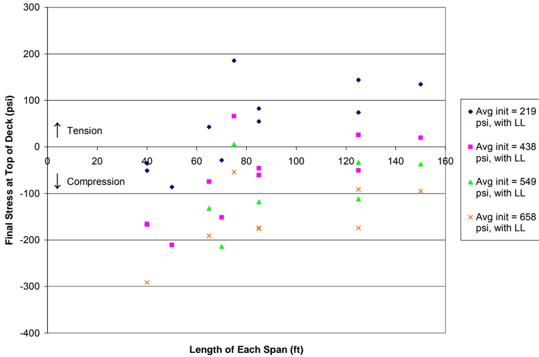
Figure 11. Final Stresses for Two-Span Continuous PCBT Girder Bridges, Incl. Live Load
