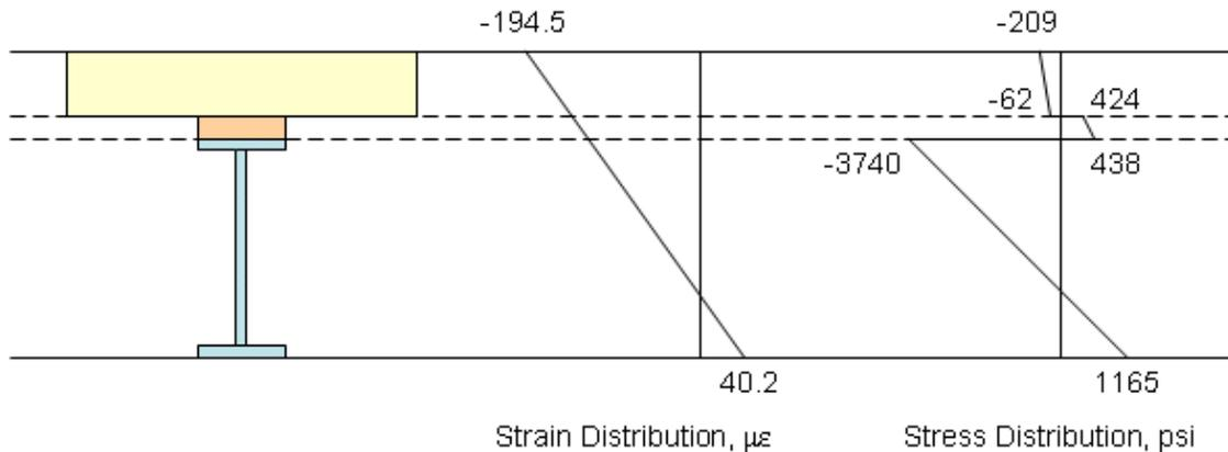
Figure 4. Typical Distributions of Stress and Strain for Steel Girder Bridge Models at End of Service Life
