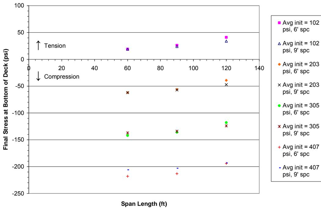
Figure 5. Final Deck Stress vs. Span Length for Simple Span Steel Girder Models
