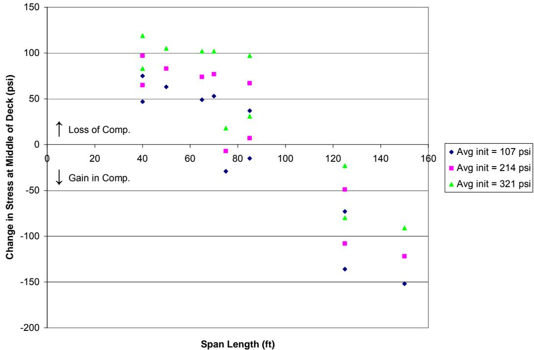
Figure 8 Net Change in Compression at Middle of Deck for PCBT Girder Models
