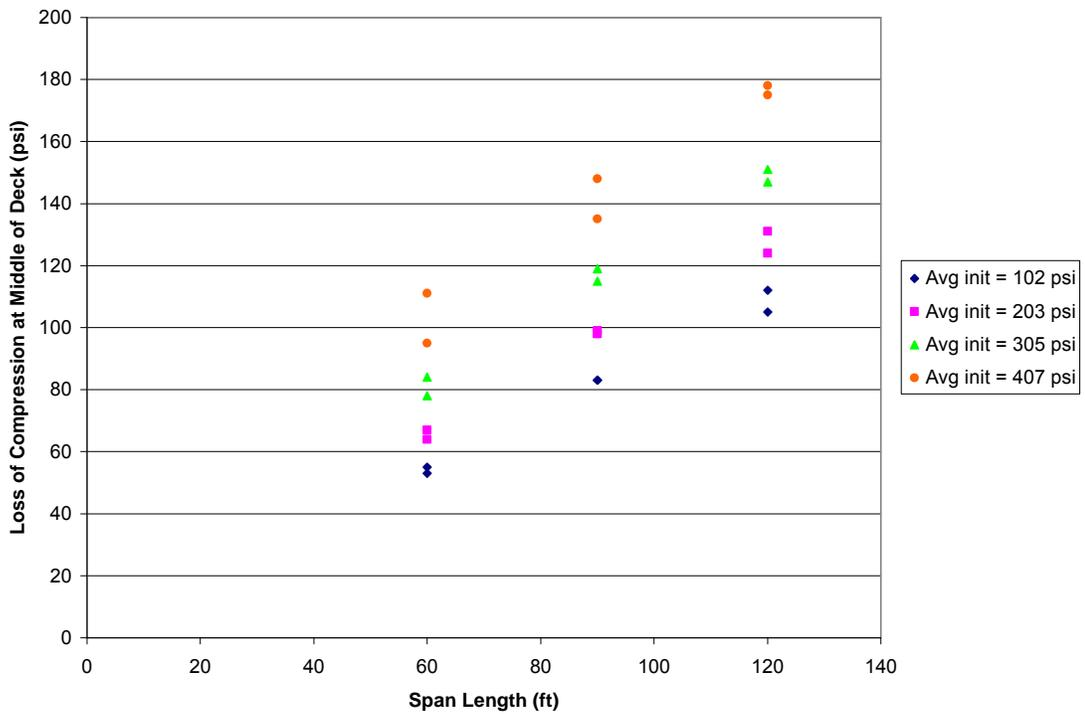
Figure 6. Net Loss of Compression at Middle of Deck for Simple Span Steel Girder Models
