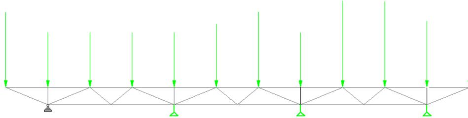
Figure 6. Strut-and-Tie Model
