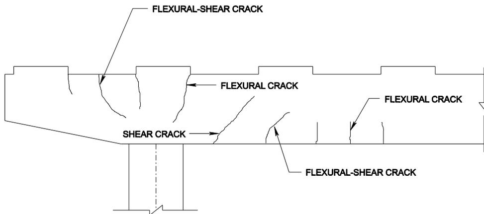
Figure 3. Typical Observed Cracks
