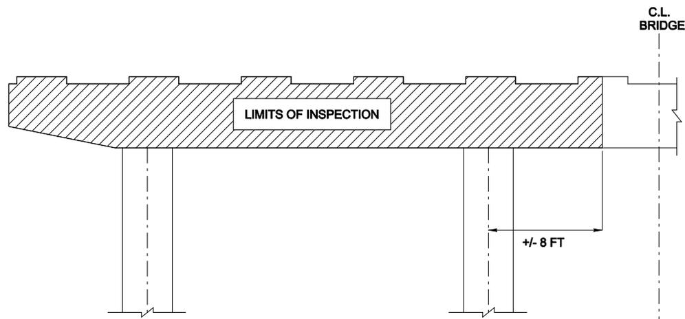
Figure 2. Limits of Inspection
