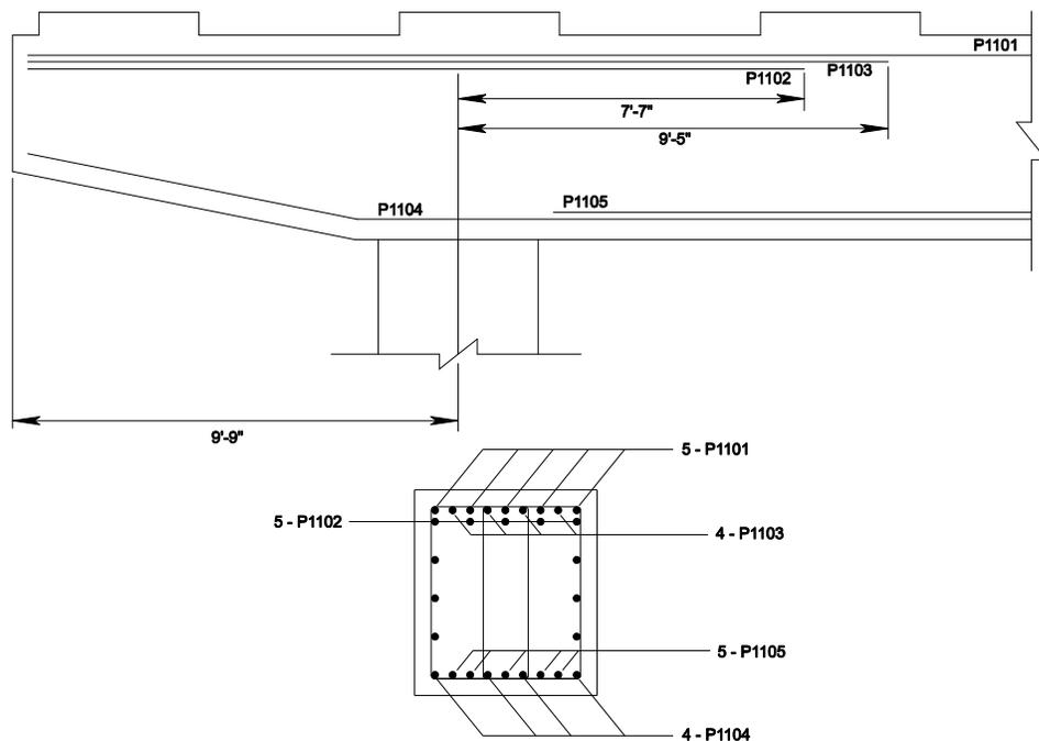
Figure 1. Typical Cap Reinforcement
