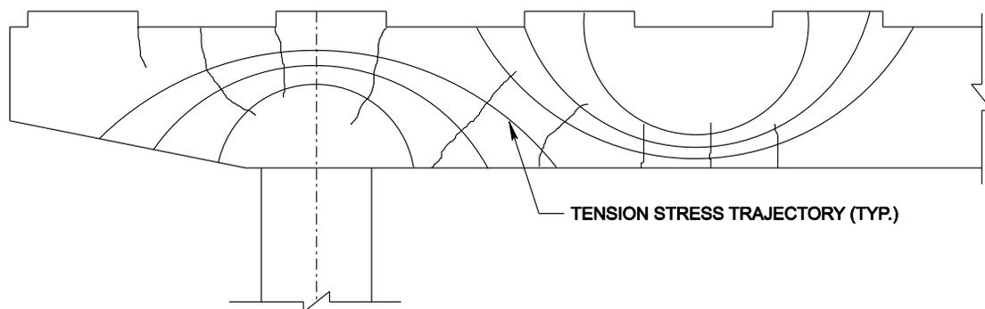
Figure 4. Principal Tension Stress Trajectories and Observed Cracks
