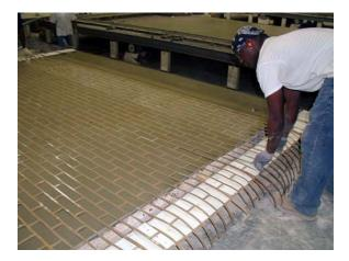
Fig. 7. Stencils are overlapped for pattern continuity
