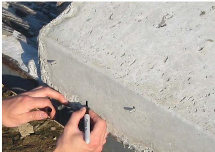
Figure 7. Strain measuring gauge points 4 ½” above bottom of girder and line for sliding
