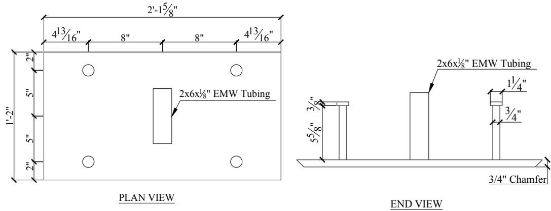
Figure 3. Drawing of embedded steel plate with 4-  $\frac{3}{4}"$  diameter studs and slot for restraining dowel.
