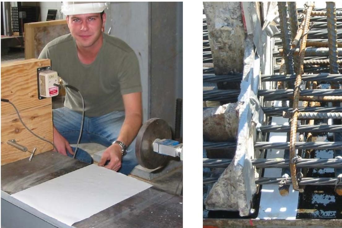
Figure 2. Teflon coated magnetic pad used in laboratory (left) and field (right).
