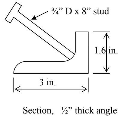
Figure 5. Embedded galvanized steel angle with two 3/4-in. diameter studs
