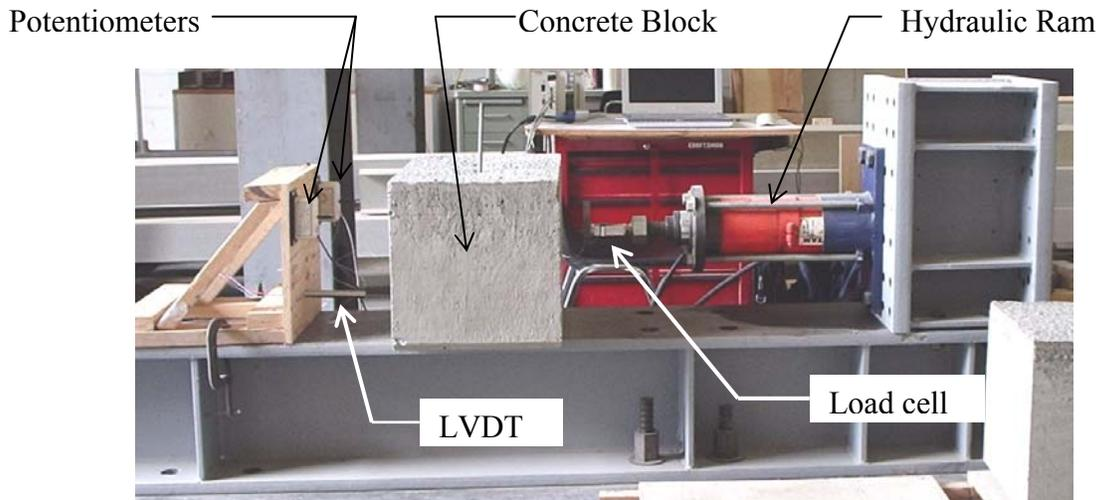
Figure 6. Laboratory sliding friction test set up.
