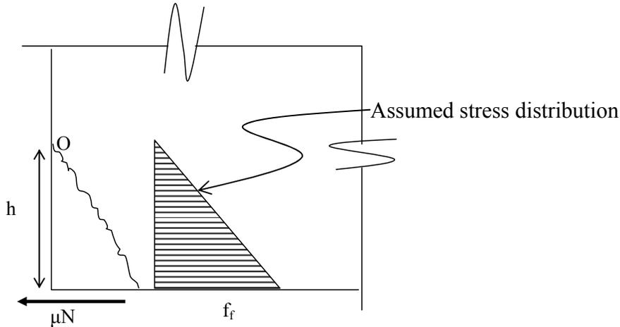
Figure 11. Schematic of cracking stresses at bottom, end of girder
