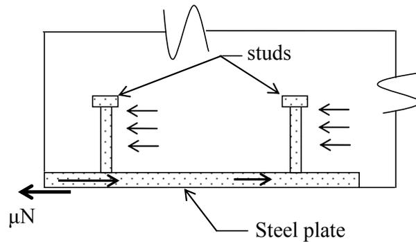
Figure 12. Schematic of tension force transfer in the embedded steel plate
