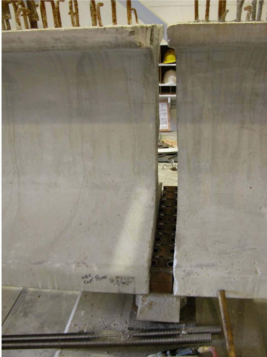
Fig.13 Confinement Steel Box Placed in Five in. Gap between Two Girders
