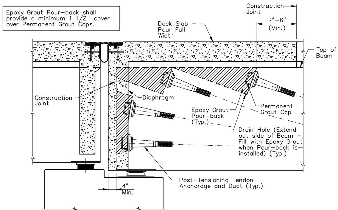
Figure 10 Details at Post-Tensioning Anchorages
