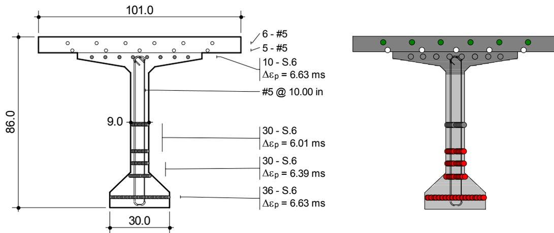
Figure 9 Example of Moment Curvature Analysis
