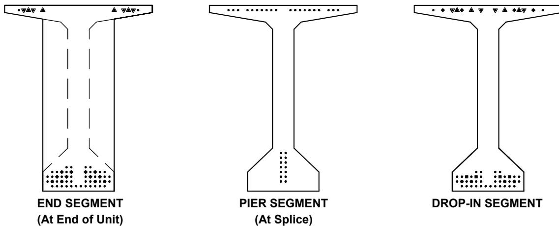
Figure 5 Pretensioned Strand Layout and Debonding
