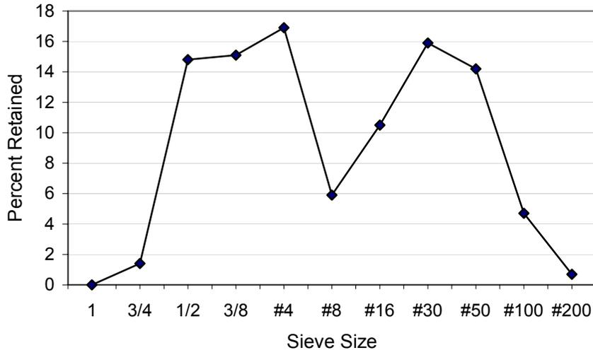
**Figure 1: Aggregate Grading**
