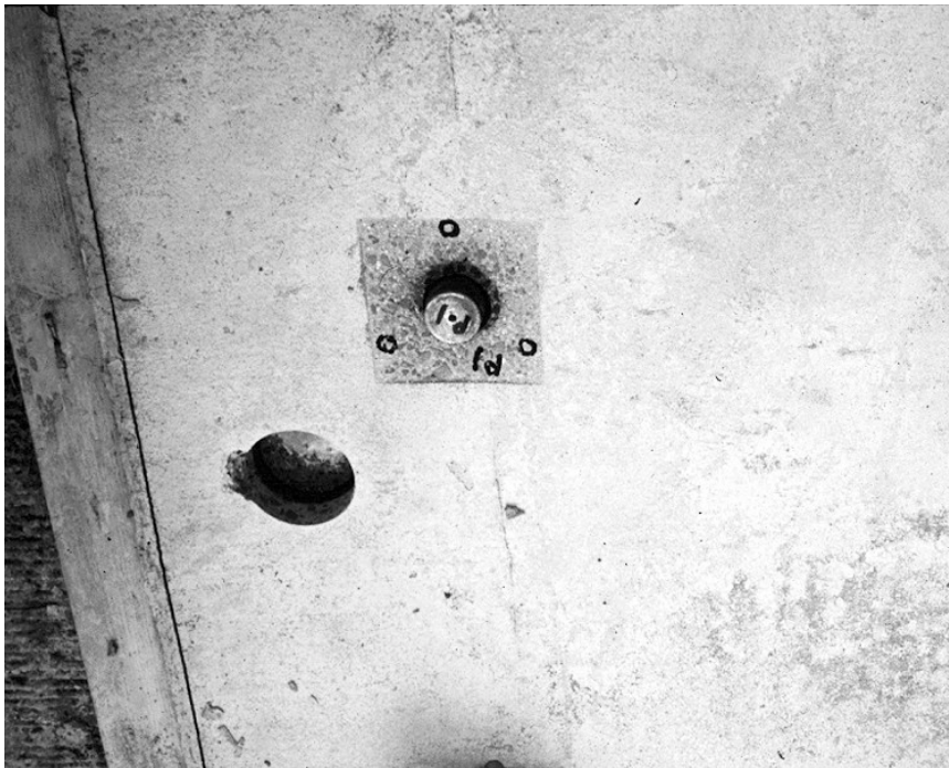
Fig. 4 Test Patch Being Tested for Tensile Bond Strength
