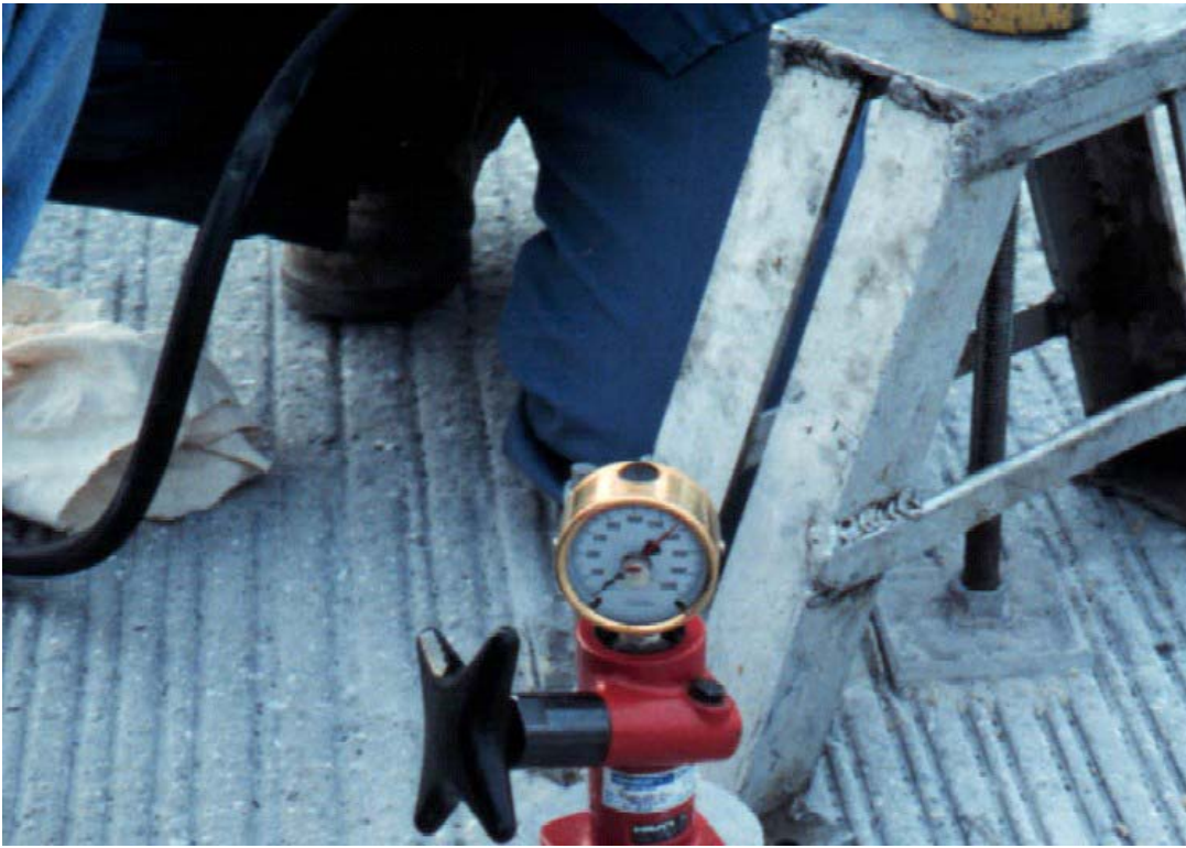
Fig. 1 Tensile Adhesion Tests on Prepared Surface Using 2-in and 4-in Square Plates
