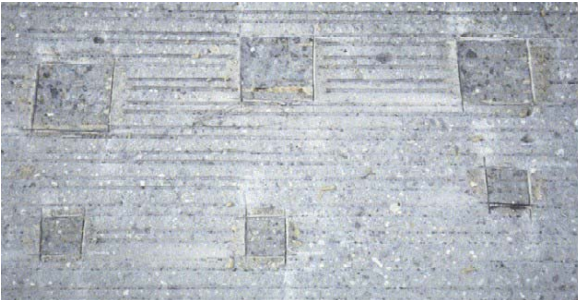
Fig. 2 Failed Surfaces Using 2-in and 4-in Square Plates
