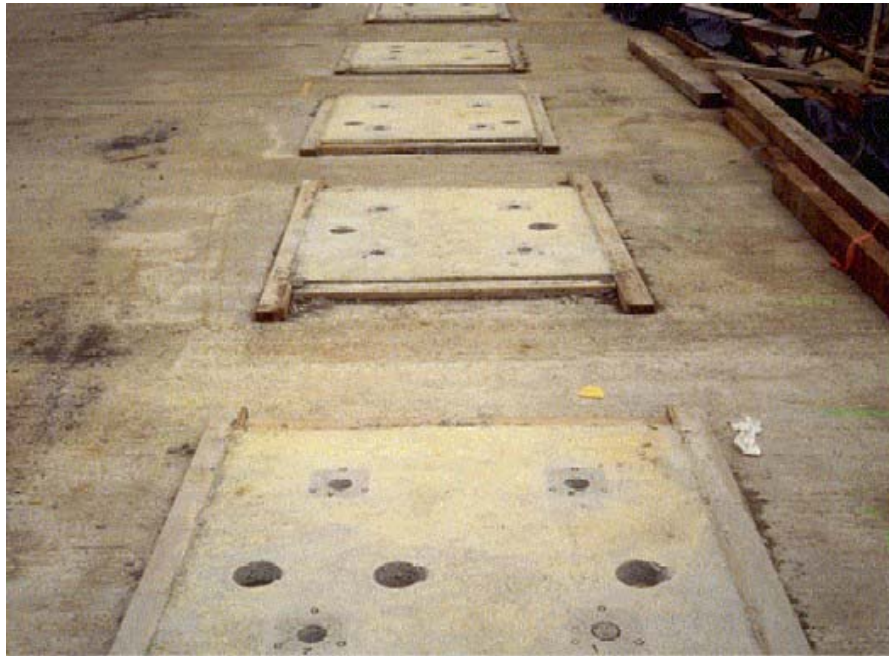
Fig. 3 HCC Overlay Test Patches with One or More Overlay Mixtures and One or More Surface Preparation Conditions
