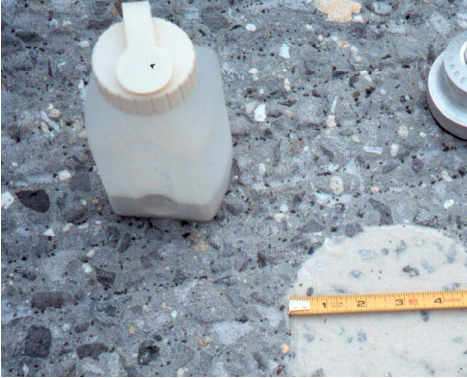
Fig. 5 Macrotexture Depth Measurement to Insure Surface Preparation, ASTM E965
