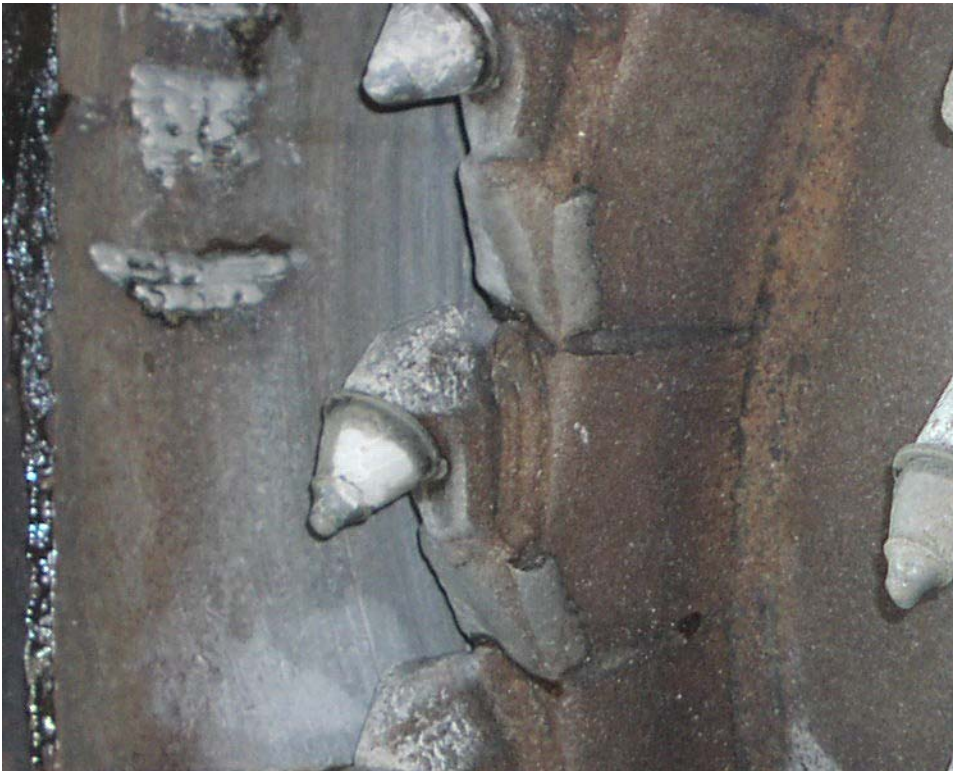
Fig. 8 Impact Heads on the Milling Machines Typically Fracture the Surface Left in Place
