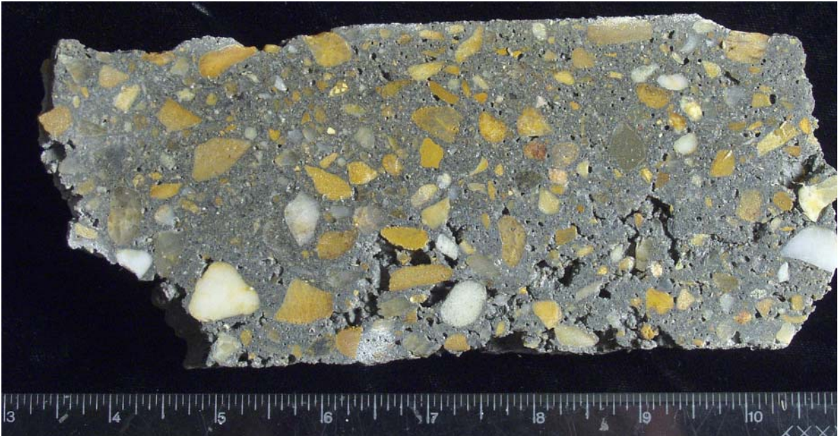
Fig. 14 The Vibrating Screed Failed to Properly Consolidate the Bottom Inch of a 3-in Thick Overlay Curing Of The Overlay Concrete
