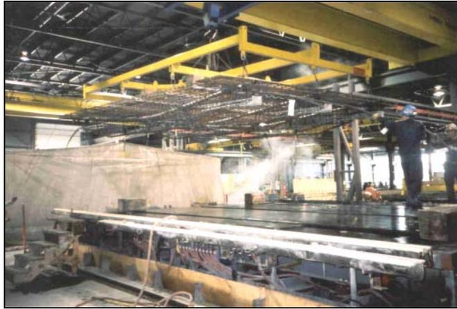
Fig. 13 Preassembled Reinforcing Steel Cages
