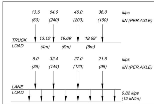
Fig. 2. QS-660 Truck Load Configuration
