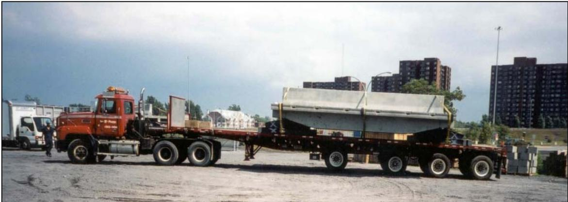
Fig. 15 Tractor-trailer Used for the Transportation of Panels
