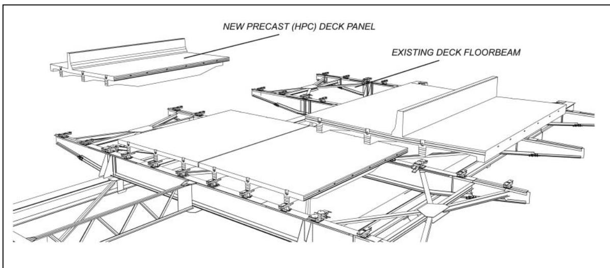
Fig. 4 Approach Span Panels Configuration
