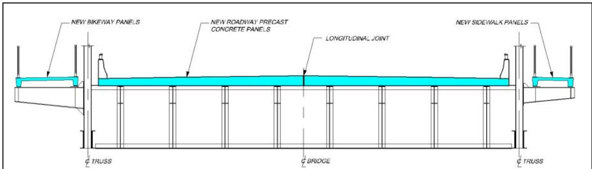
Fig. 11 Typical Cross-Section
