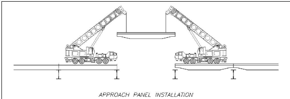
Fig. 16 Set-up for Removal and Installation of New Deck Panels
