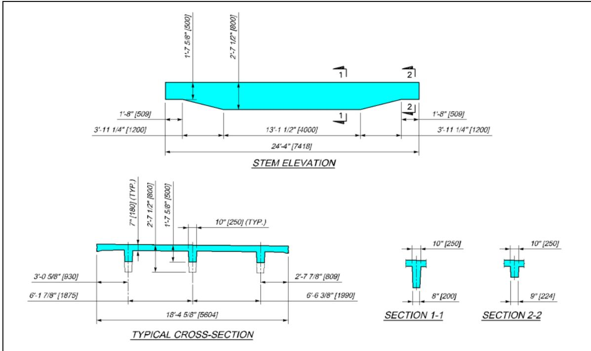
Fig. 5 Typical Approach Span Deck Panel
