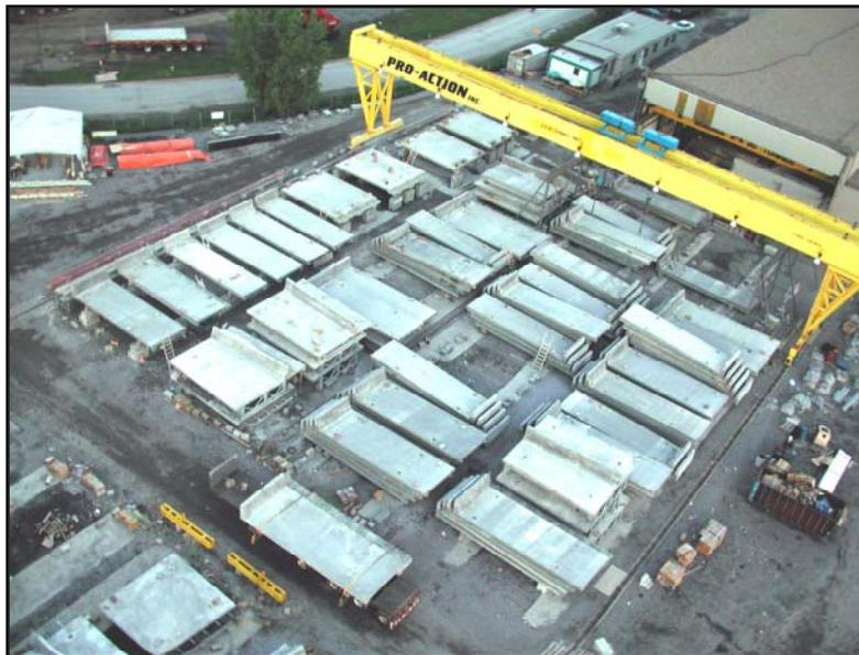
Fig. 12 Storage Yard and Stockpile of HPC Precast Prestressed Panels
