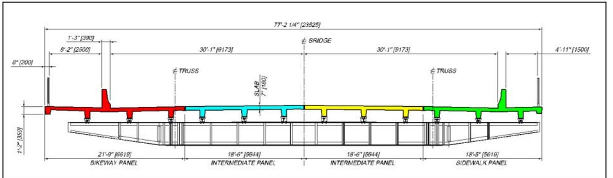
Fig. 3 Approach Span – Typical Deck Cross-Section
