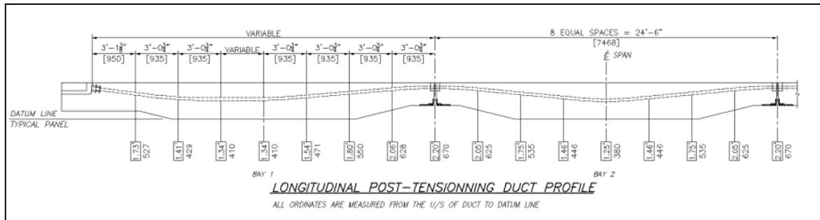
Fig. 19 Longitudinal Post-tensioning Duct Profile
