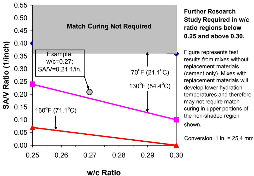
Figure 8. Guideline for Selecting Critical SA/V Ratio for Using Match Curing Technology for Design Compressive Strength
