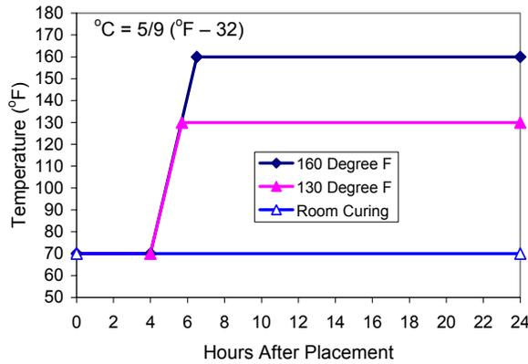
Figure 2. Accelerated Curing Temperature Profiles
