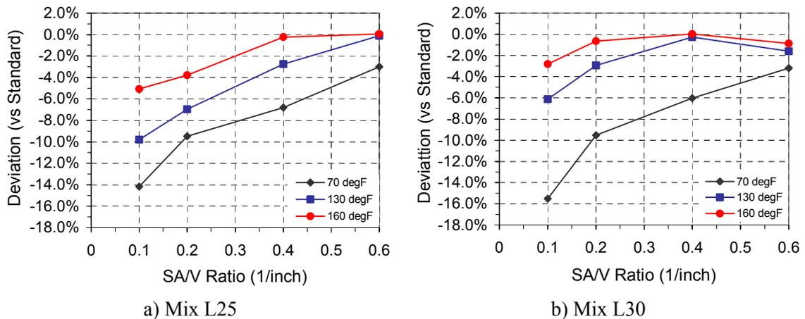
Figure 7: Deviation of Match-cured Specimens from ASTM Member-cured at Later-Age (56 days)
