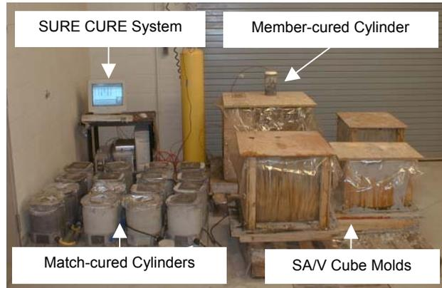
Figure 3. Test Setup in the Room Condition
