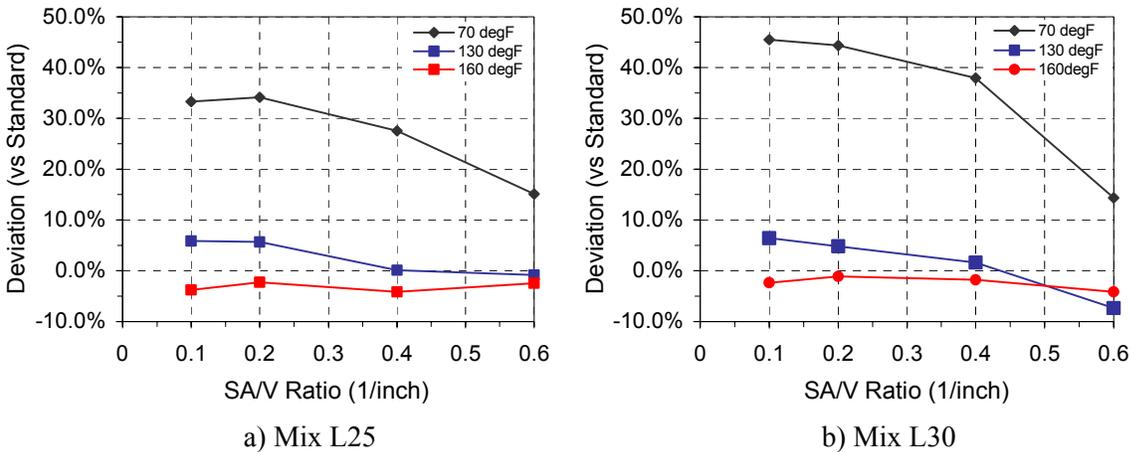
Figure 6: Deviation of Match-cured Specimens from ASTM Member-cured at Early-Age (1 day)
