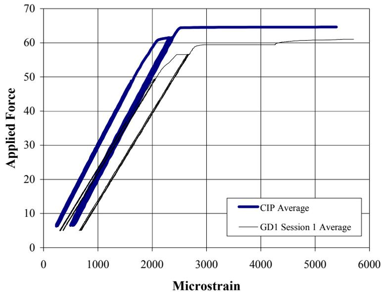
Figure 17 CIP1 and GD1 Applied Force vs. Strain at Bar Lead
