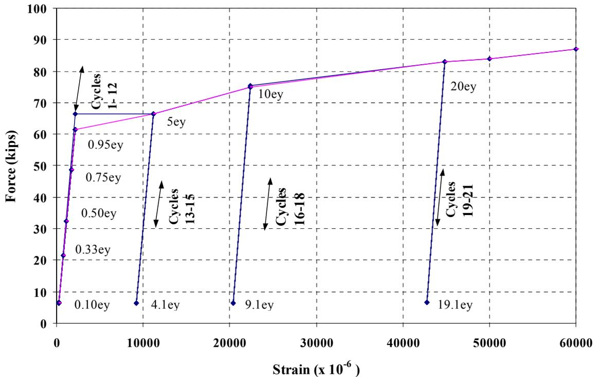
Figure 8. Bar Force vs. Bar Strain for Tension Cycles
