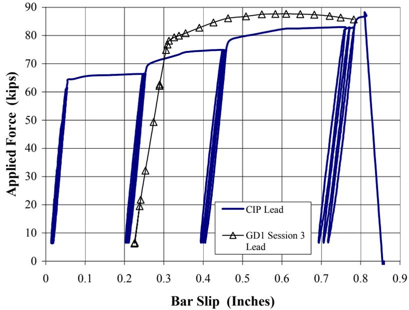
Figure 16 CIP1 and GD1 Applied Force vs. Bar Slip at Bar Lead
