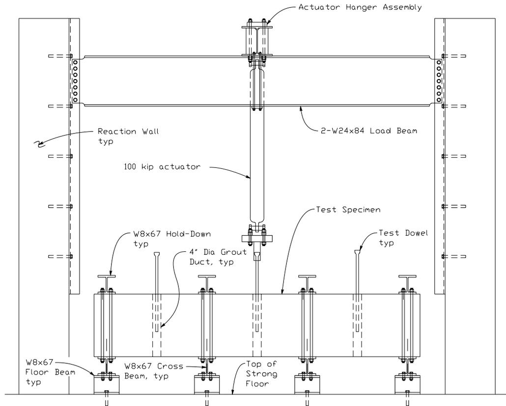
Figure 9. Test Setup Elevation
