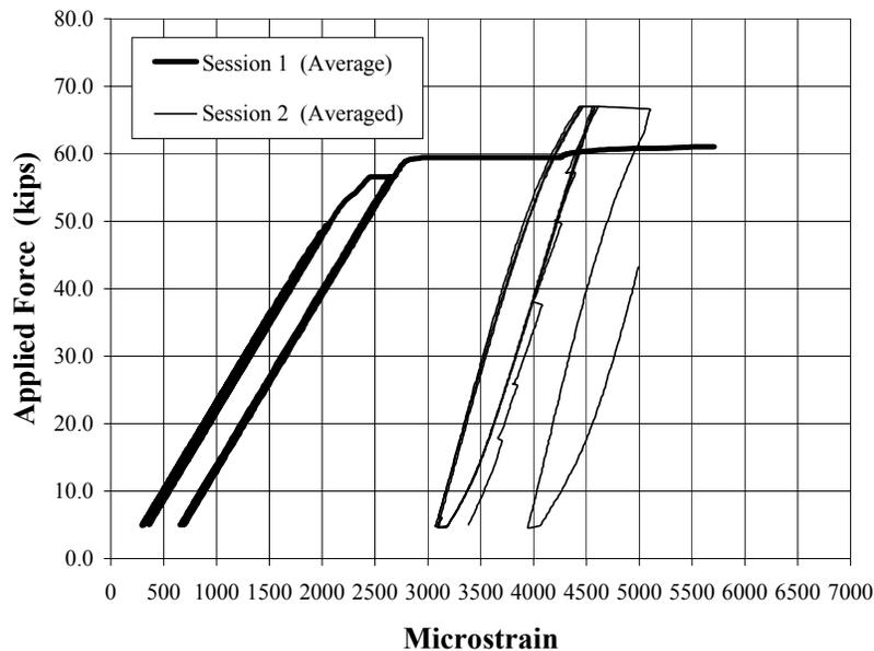
Figure 12. GD1 Applied Force vs. Strain at Bar Lead
