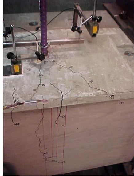
Figure 11. GD1 Crack Pattern
