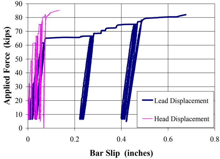
Figure 14. GD2 Applied Force vs. Slip at Bar Lead
