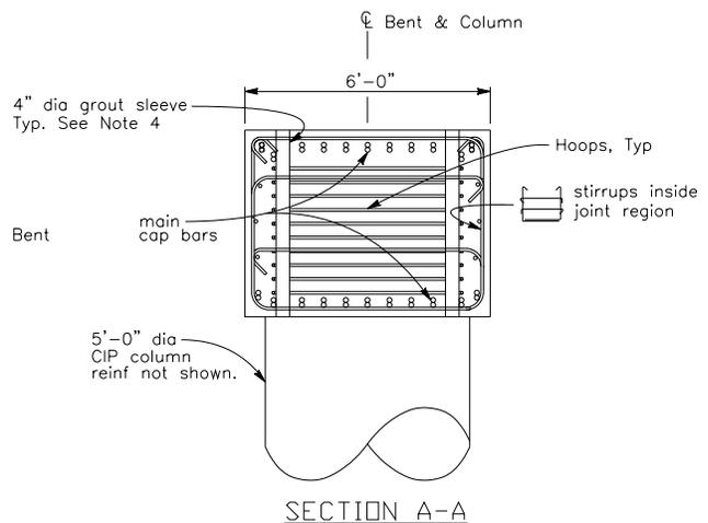
Figure 2. Section through Bent Cap at the Connection
