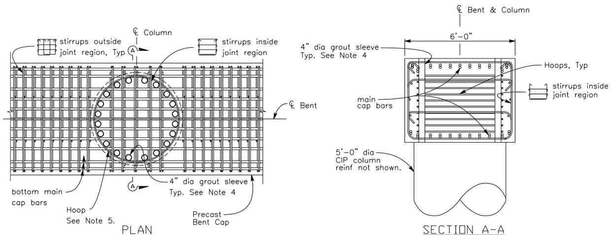
Figure 1. Reinforcement Plan for Moment Connection
