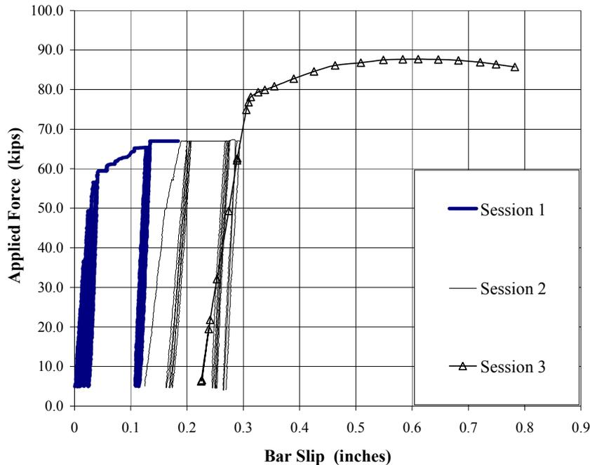
Figure 13. GD1 Applied Force Vs. Bar Slip at Bar Lead
