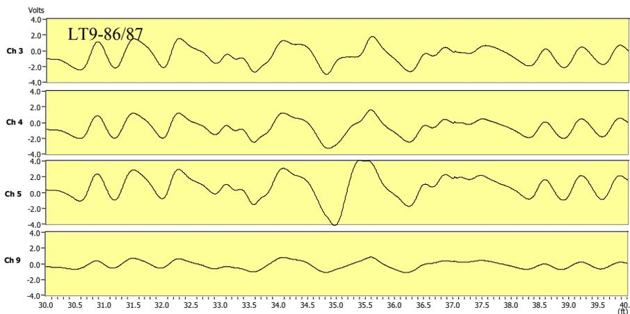
Figure 18 - MFL signals (4 channels) for tendon # 9 between segments 86 and 87 (data for 5 feet of the tendon on both sides of the joint between segments 86 and 87)
