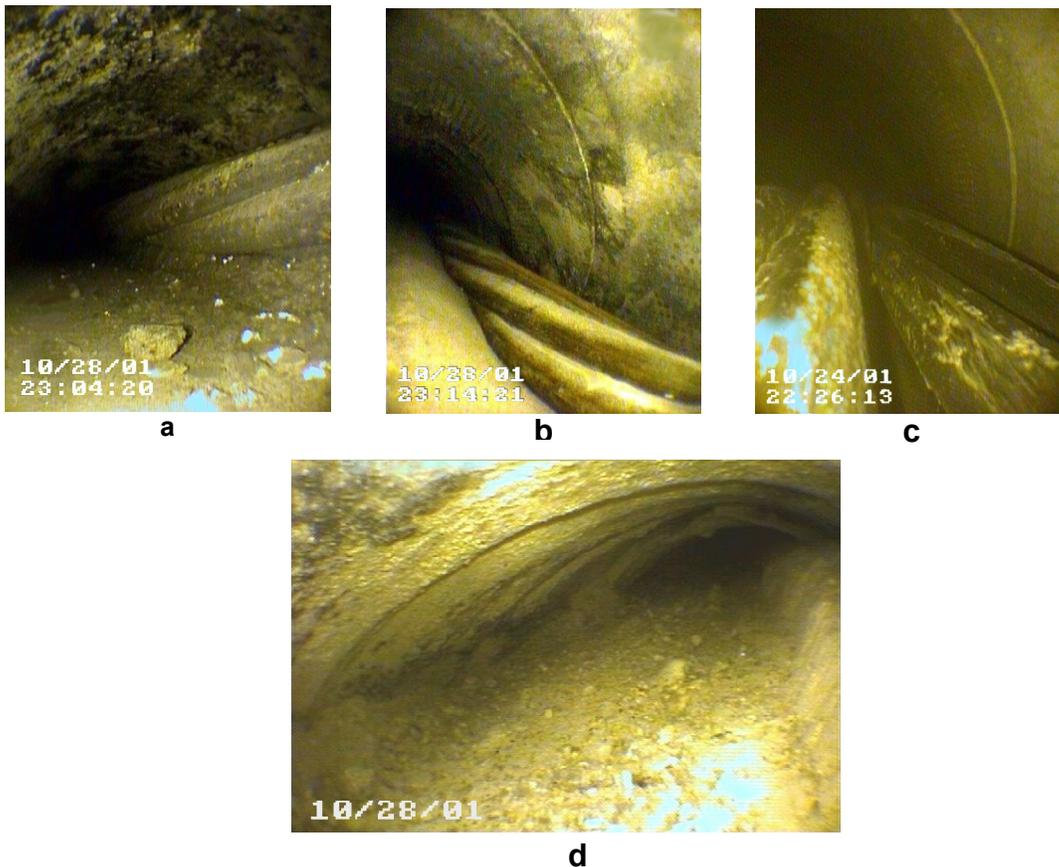
Figure 5 – Photos a and b show duct partially grouted with strand exposure. Photo c shows voided duct with strands fully exposed. Photo d shows partially grouted duct, no strands exposed.
