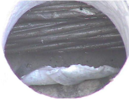
Figure 15. Tendon No. 10, core drilled at segment No. 54.
