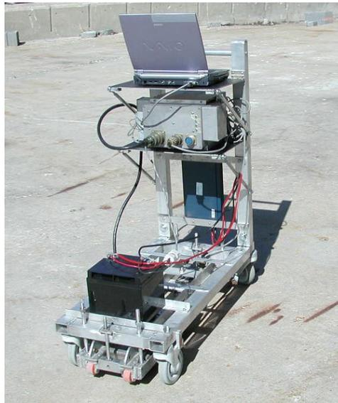
Figure 16 – Photograph of the MFL equipment as configured for testing internal P-T tendons in a bridge deck
