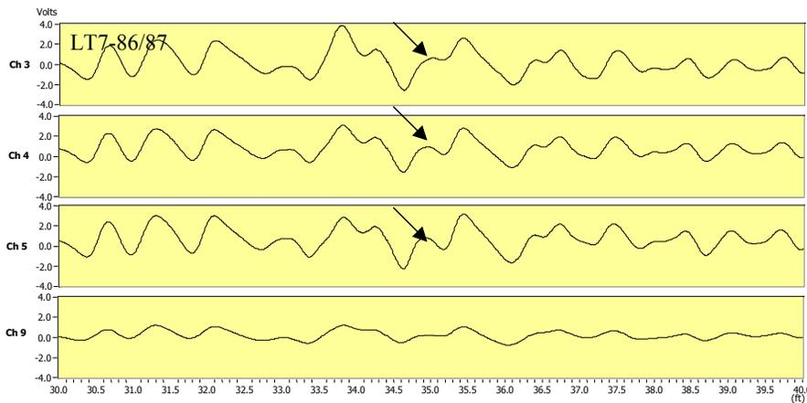
Figure 17 - MFL signals (4 channels) for tendon # 7 between segments 86 and 87 (data for 5 feet of the tendons on both sides of the joint between segments 86 and 87)
