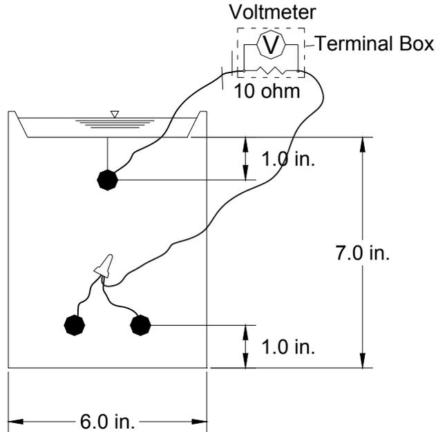
Fig. 3 Test Specimen for Cracked Beam Test<sup>4</sup>
