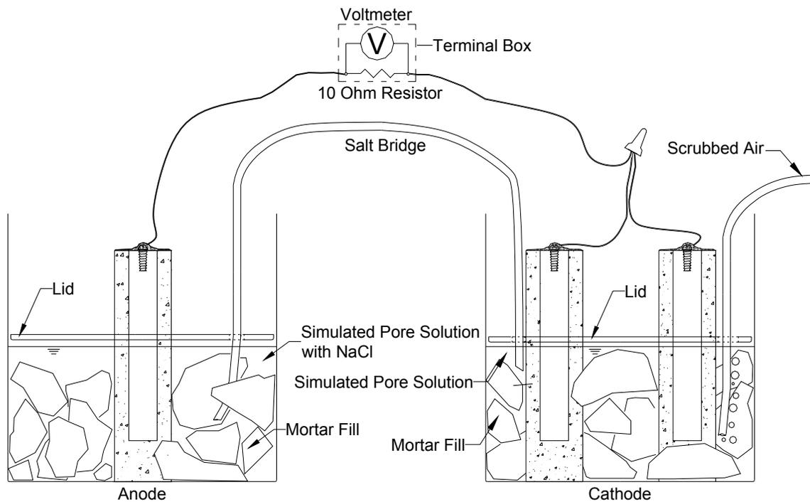
Fig. 1 Schematic of Macrocell Test<sup>4</sup>
