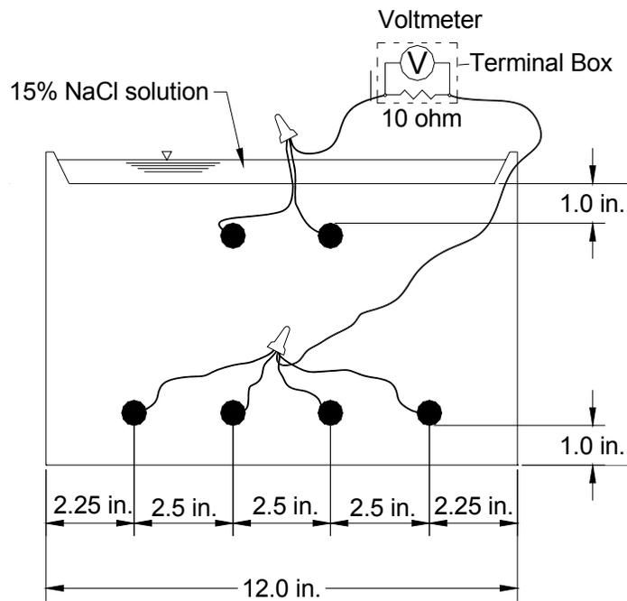
Fig. 2 Test Specimen for Southern Exposure Test<sup>4</sup>
