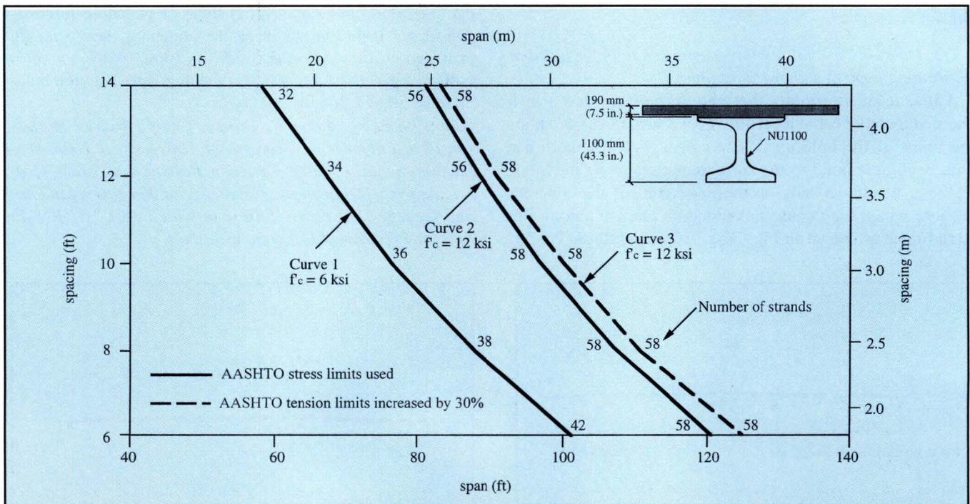
Fig. 4. Impact of using HPC on simple span capacity of NU1100 I-girder bridge.
