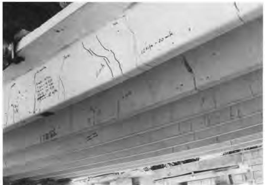
Fig. 16. Crack pattern at ultimate load.
