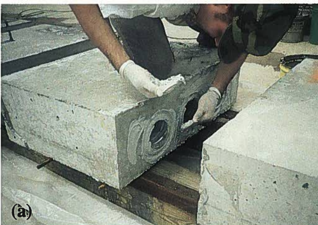
Fig. 4. Details of epoxy application: (a) Epoxy application on annulus and one face; (b) Epoxy application in a typical top strip.
