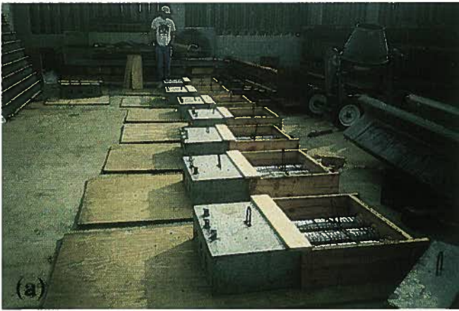
Fig. 3. Details of test setup: (a) Layout of casting cells in yard; (b) Assembly setup for the model segmental beams.
