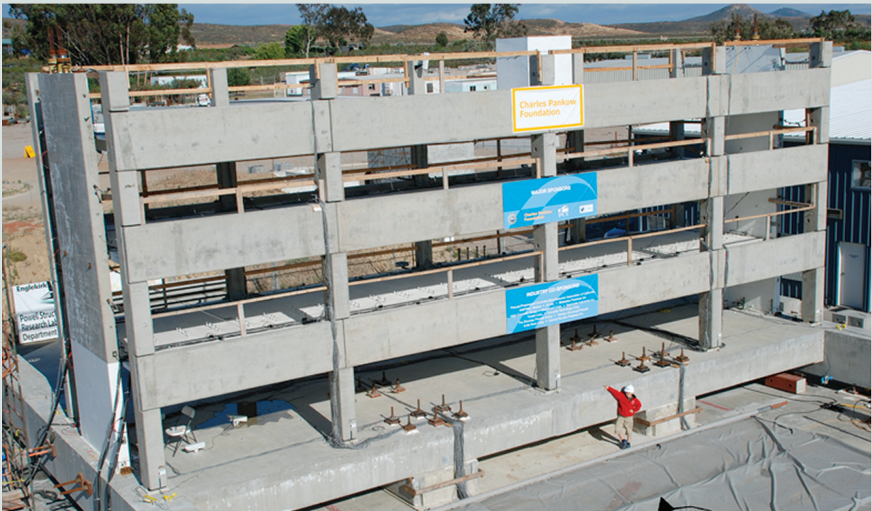
Three-story, half-scale precast concrete structure on the shake table. Source: Schoettler et al. (2009).
