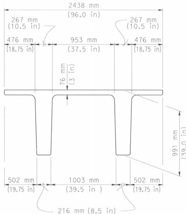
Fig. 6 Proposed Dimensions of Non-Standard Double Tee Girder.
