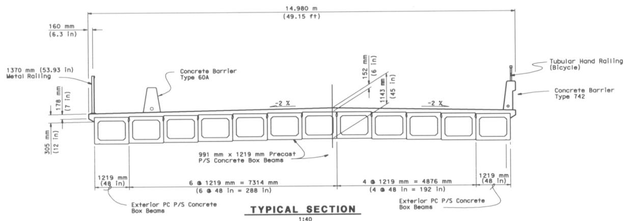
Fig. 3 Typical Cross Section – Original Design.
