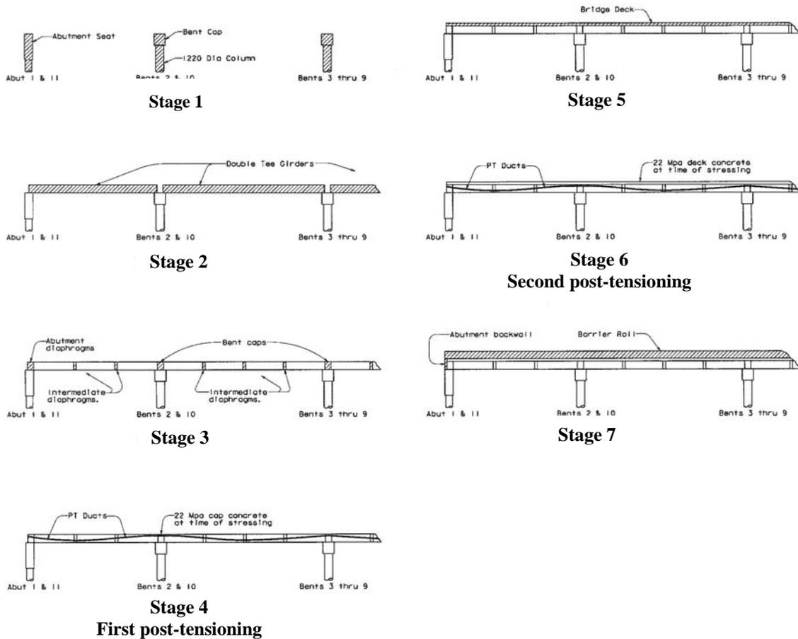
Fig. 7 Sequence of Construction Stages
