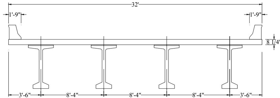
Fig. 1. Typical Cross Section of Prestressed Concrete Bulb-Tee Girder Bridge
