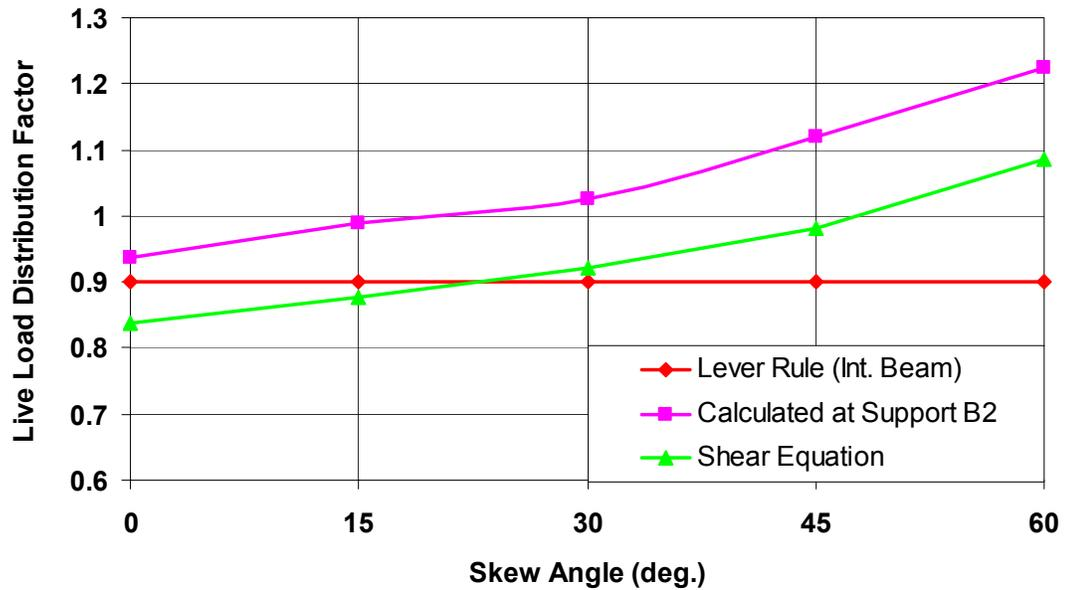
Fig. 11. Comparison to the Current Procedures (Interior Beam)
