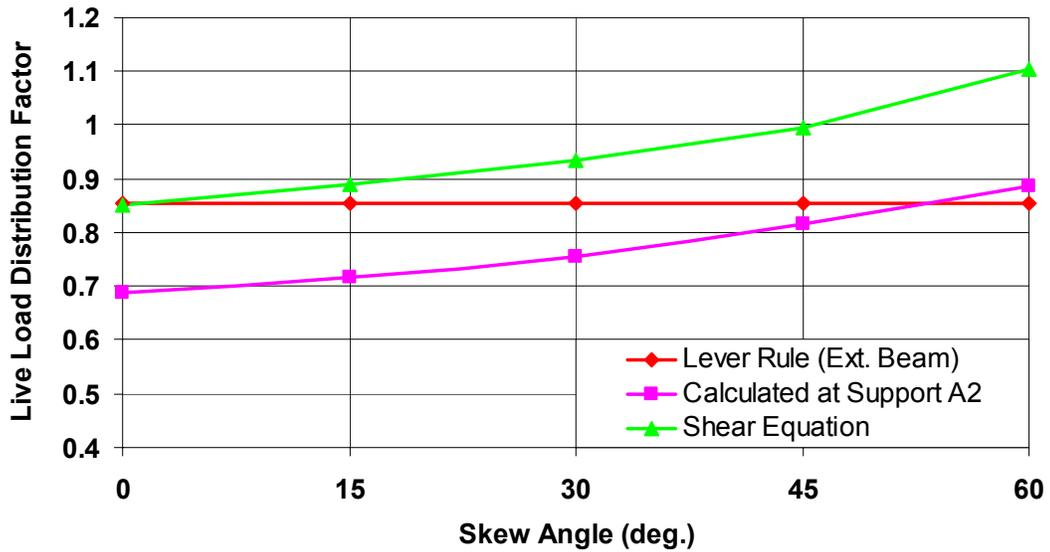
Fig. 10. Comparison to the Current Procedures (Exterior Beam)
