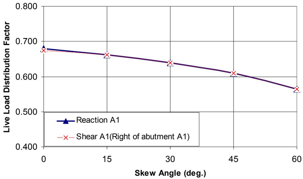
Fig. 6. Distribution Factors of Reaction and Shear at Support A1
