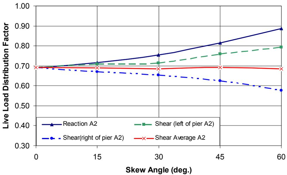
Fig. 7. Distribution Factors of Reaction and Shear at Pier A2
