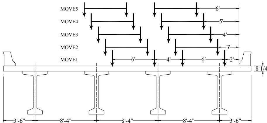
Fig. 4. Loading Positions for Two Lanes Loaded
