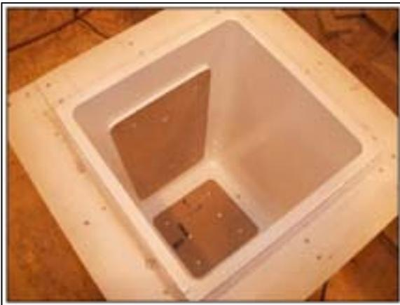
Fig. 13 Inside of mould, showing openings for the top and rear doors
