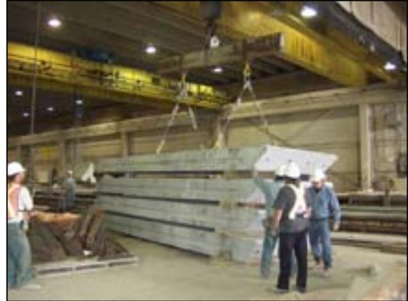
Fig. 7 Stack casting for 48 h thermal treatment
