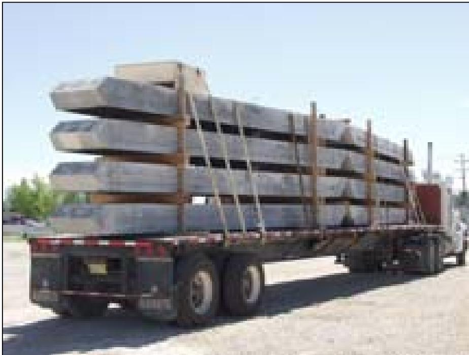
Fig. 8 Trucking eight panels per truck
